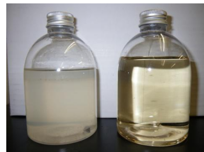
Fig. 13: On the left side, there is a bottle of untreated greywater visible. On the right side, there is a sample of purified greywater. It is clear and has no visible residues. The light brown colour is caused by humins.
