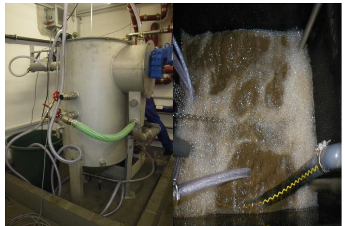
Fig.7: Left: Stainless steel tank (cylinder) includes pre-treatment. Right: This is how the MBR looks like about three quarters filled up with activated sludge. The bubbles are produced by air that is blown into the reactor at the bottom of the container.
