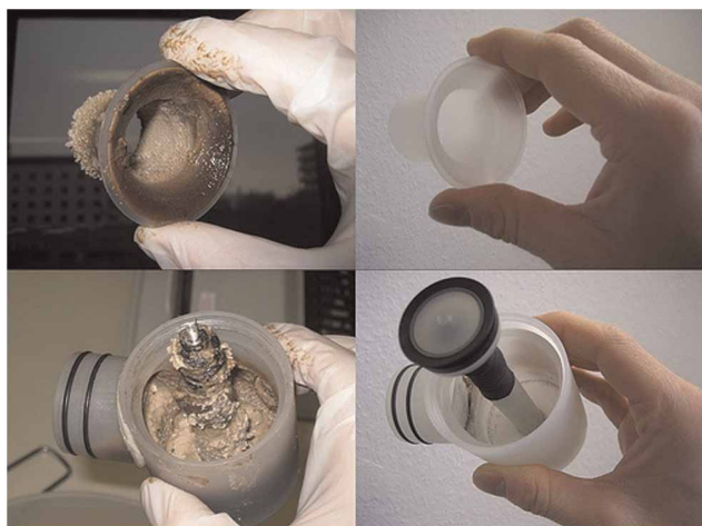
Figure 5 | Left: Soft urine precipitations inside a urine valve (of 'NoMix toilet' by Roediger Vacuum GmbH). Right: the same valve after cleaning by soaking in citric acid for several days (source: L. Ulrich, 2009).
