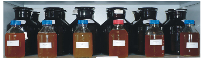
Bottles for storage experiment (background) and transparent reference bottles for inspection of optical appearance
