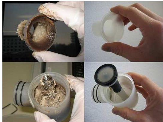
Figure 5: Left: Soft urine precipitations inside a urine valve. Right: the same valve after cleaning soaking in citric acid for several days (source: L. Ulrich, 2009).
