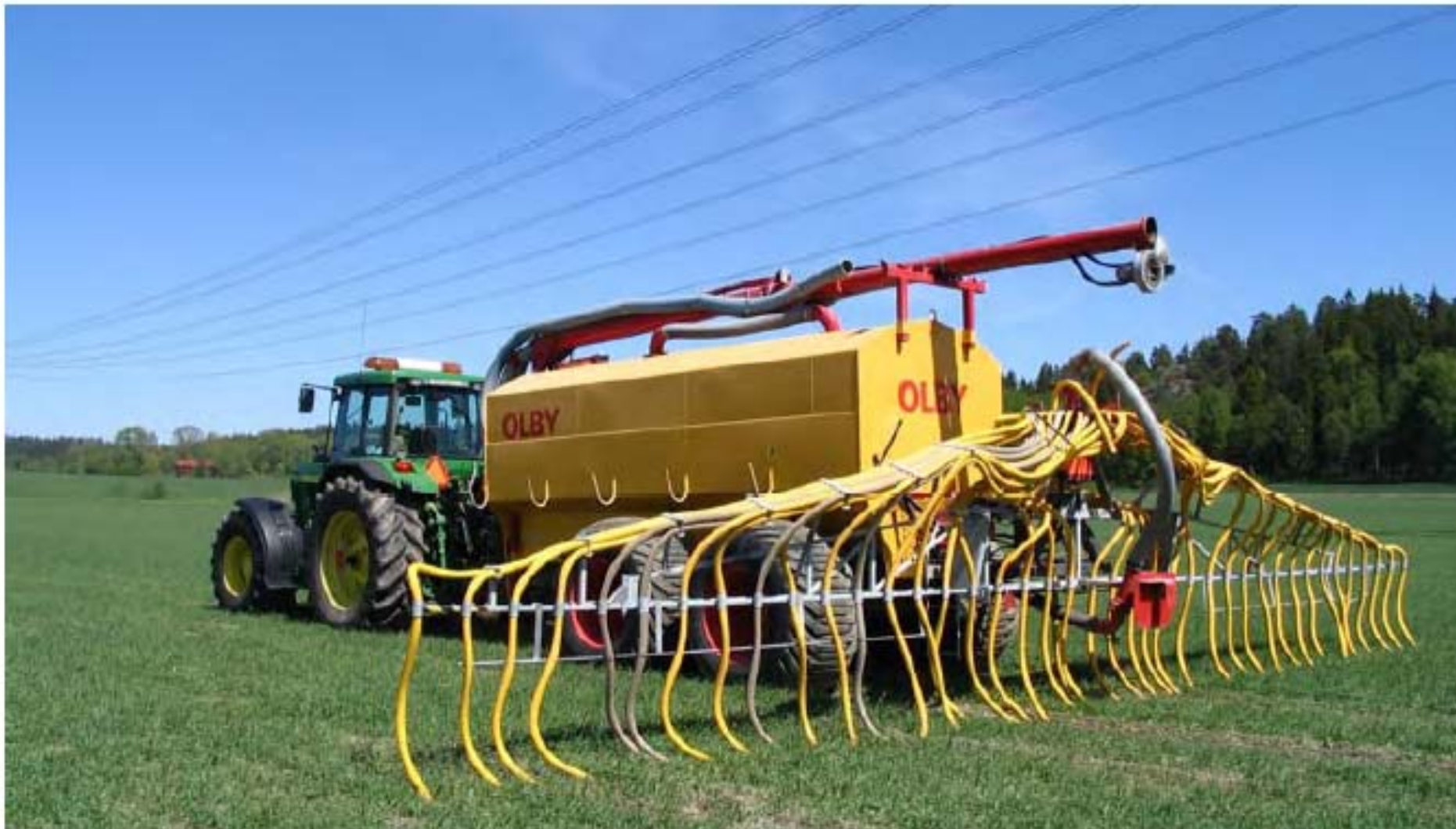
Figure 21. Large scale application of urine using a slurry spreader with trailing hoses. Photo: Mats Johansson.
