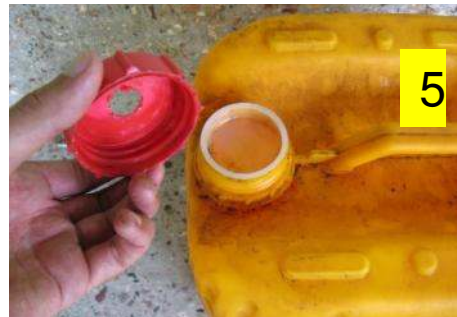
5 Cut hole into cap, not into removed plug
