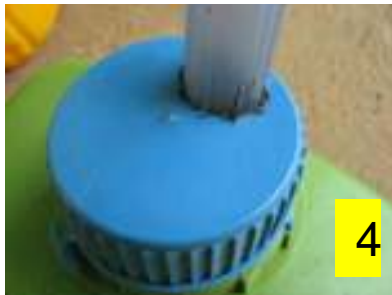
4 Cut hole into cap, insert hose, attach with glue/silicon
