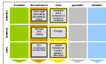
Fig. 2: Applied sanitation components in this project
