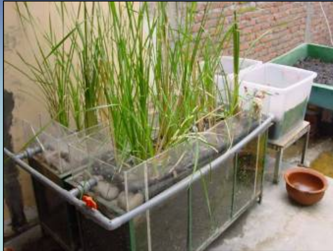
Small scale constructed wetland
