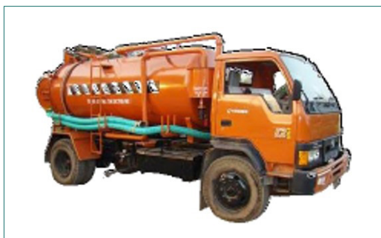
Figure 19: Truck mounted tanker
