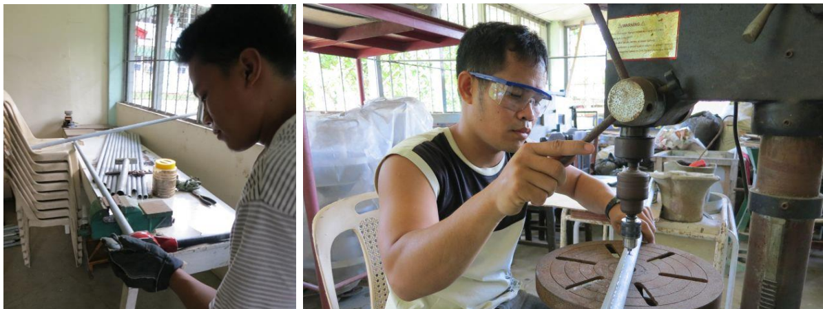
Figure 11: Production Process at ATC. Cutting threads with die and drilling bore holes
