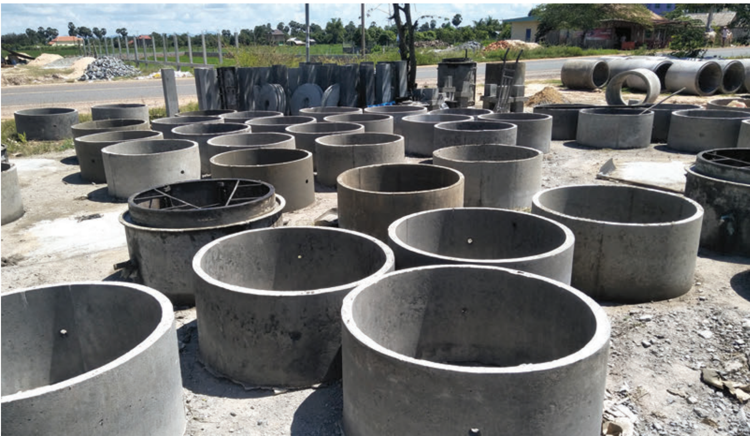
Concrete rings used in the construction of latrines.
