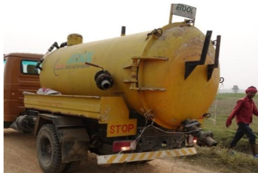
Figure 6: Truck mounted vacuum tanker (Source: Aishwarya/CSE, 2016)
