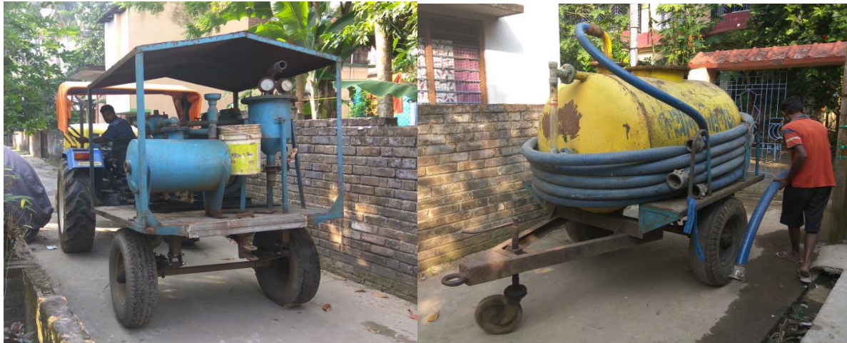
Figure 9: Smaller vacuum tanker with generator in narrow lanes (Source: Aishwarya/CSE, 2016)
