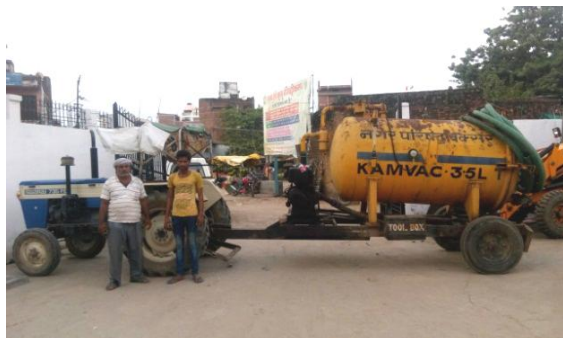
Figure 1: Tractor mounted vacuum tanker (Source: Amrita/CSE, 2016)
