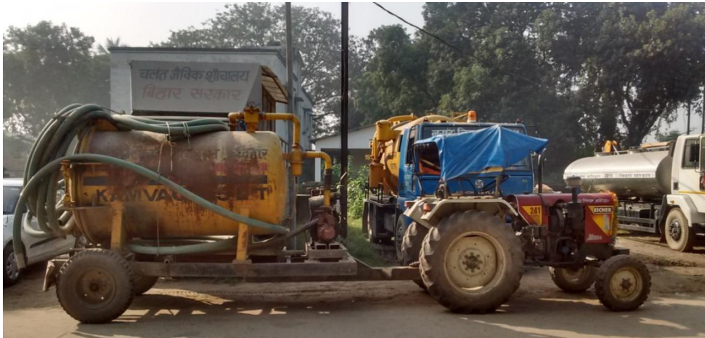
Figure 7: Tractor mounted tanker at KMC (Source: Anshul/CSE, 2016)
