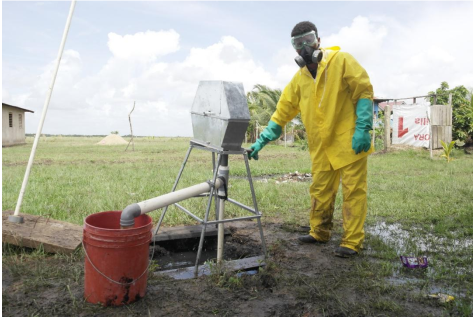
Figure 8: Demonstration of rope pump prototype for extraction of faecal sludge from on-site septic tanks. (WaterAid/Eduardo Rodriguez, 2017)
