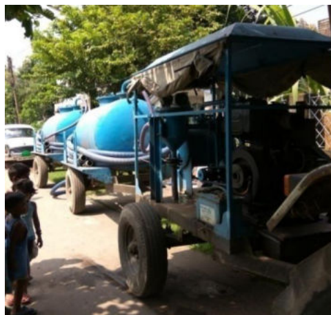
Figure 6: Suction pump of 5HP assembled with the tanker (Source: Anil/CSE, 2016)
