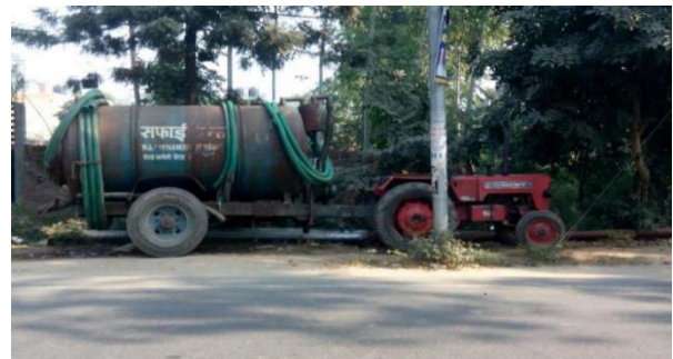
Figure 3: Vacuum tanker (5,000 litres capacity) used for emptying of OSS (Source: Amrita/CSE, 2016)
