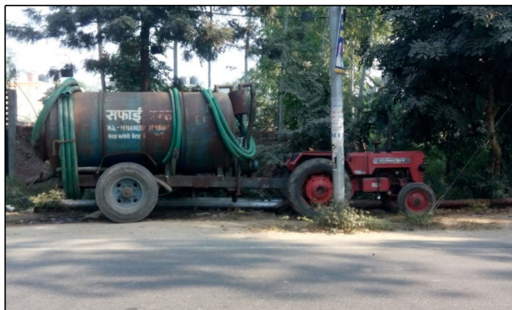
Figure 5: Vacuum tanker (4,000 litres capacity) used for emptying of OSS (Source: Amrita/CSE, 2016)
