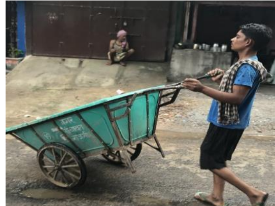
Figure 9: Cart used to transport faecal sludge emptied by manual scavengers (Harsh/NU/2019).
