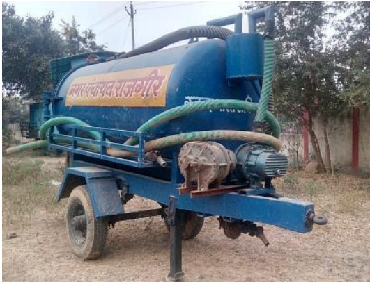
Figure 8: NPR desludging vacuum tank standing in the NPR store area (Gayatri/Nu/2019).
