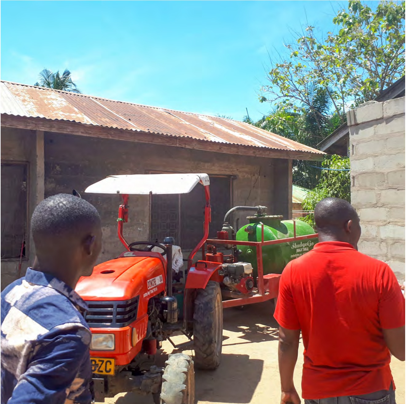
Figure 15: Sludge-Go emptying technology
