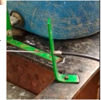
Tap is controlled by the foot pedal through a brake wire .
