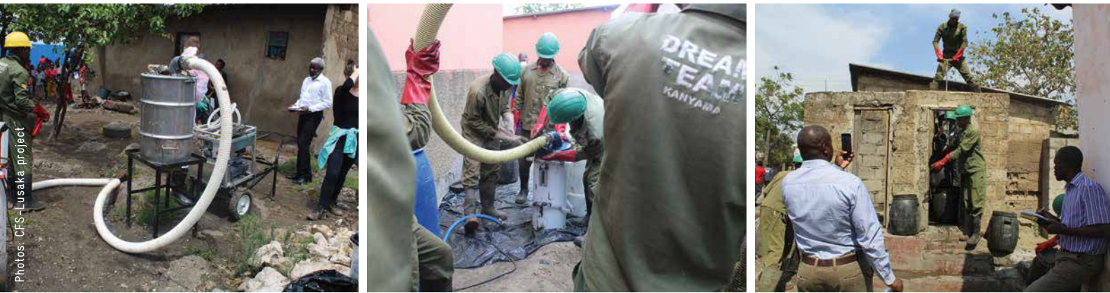
From left to right: The Flexcravator, the eVac, and the Gulper being tested in Lusaka
