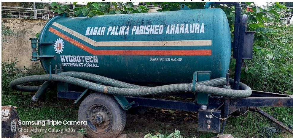
Figure 3: Government Desludging Tanker of Capacity 5kl (Manish/CSE,2020)
