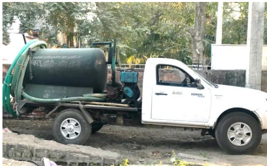
Figure 9: Vacuum Trucks 1500 L and 600 L owned by JNN (Source: Shrutaswinee/CSE, 2020)
