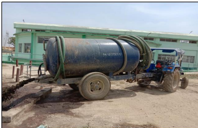
Figure 3: PTO tanker-mounted tractor (Source: Apurva/PSI,2020).
