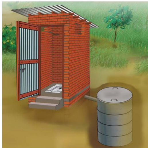
Figure 4: Illustration of an off-set toilet with one pit (Source: (SNV Nepal, Jawalakhel, Lalitpur, 2017)).
