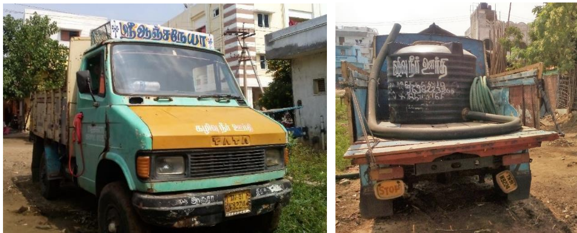
Figure 2.1: An Early Form of Mechanical Emptying Truck in Trichy
