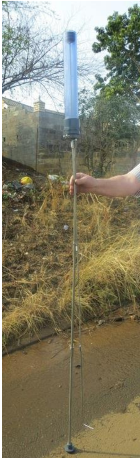
FIGURE H.4. SAME SAMPLING TUBE AS BEFORE, WITH LONG HANDLE IN VIEW. THE HANDLE CONSISTS OF SEVERAL SMALLER PIECES FITTED TOGETHER TO ALLOW THE LENGTH TO BE ADJUSTED AS NEEDED
