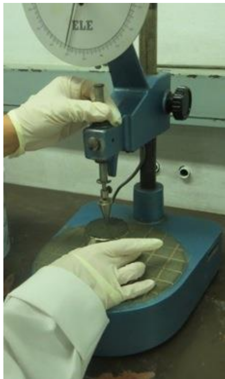
FIGURE C.4. PREPARING APPARATUS TO PERFORM THE TEST. THE CONE MUST JUST SCRATCH THE SURFACE OF THE SLUDGE IN THE CUP
