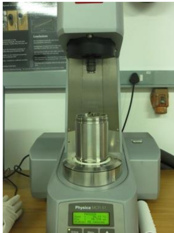
FIGURE D.2. THE CYLINDER CONTAINING THE SAMPLE IS SCREWED INTO PLACE ON THE RHEOMETER
