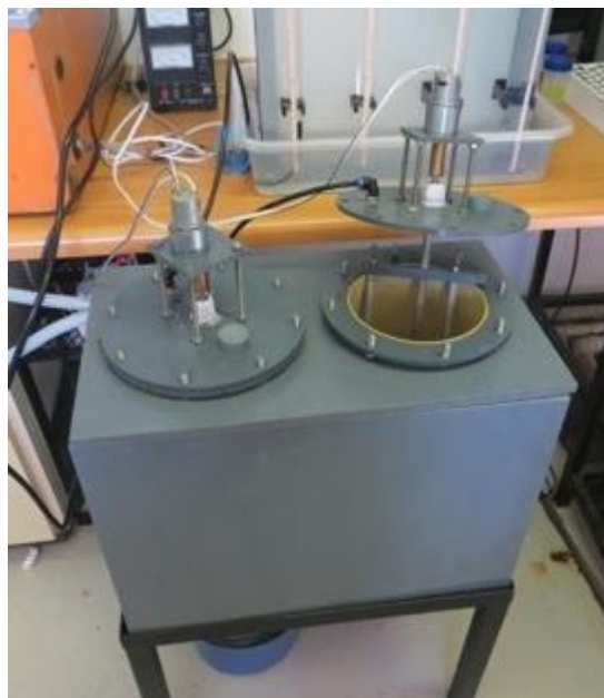
FIGURE E.2. THE INTERIOR OF THE TANK AND THE STIRRER
