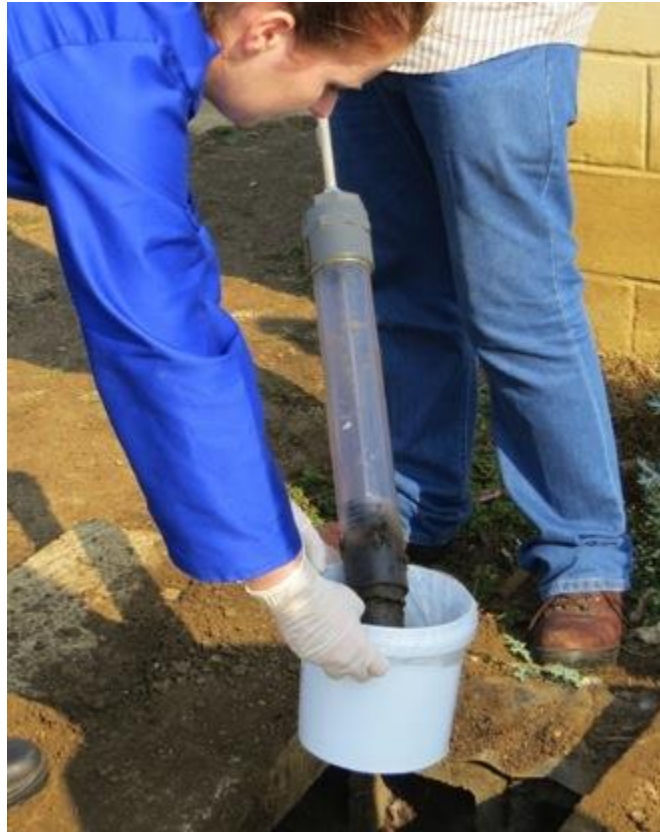
FIGURE H.7. SLUDGE BEING PUSHED OUT OF SAMPLER INTO THE STORAGE CONTAINER USING THE INTERNAL BUNG
