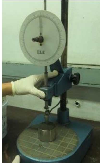
FIGURE C.5. THE BUTTON IS PRESSED FOR 5 SECONDS TO RELEASE THE CONE INTO THE SLUDGE
