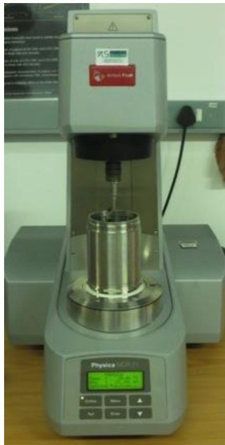
FIGURE D.4. THE VANE IS MECHANICALLY LOWERED INTO THE SLUDGE AND THE TEST BEGINS, THE DATA BEING RECORDED AND STORED BY THE COMPUTER
