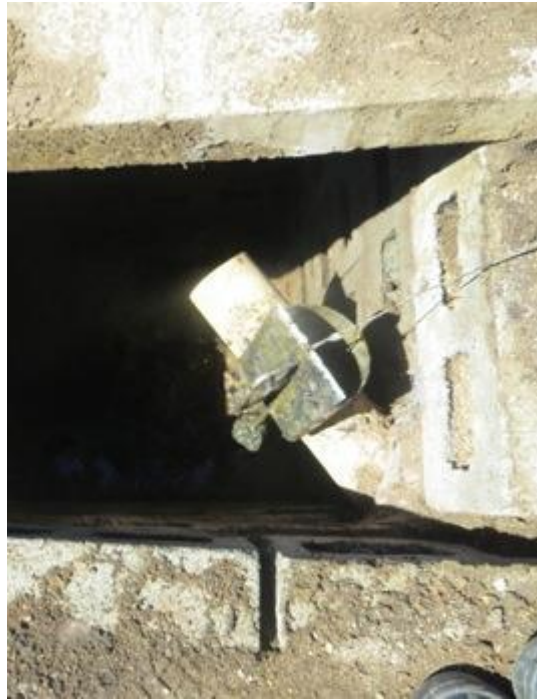
FIGURE H.10. THE BASE OF THE BUCKET CAN MOVE, A WEIGHT WAS ADDED TO EXTERIOR OF BASE TO HELP PUSH THE SLUDGE OUT OF THE BUCKET INTO THE SAMPLING CONTAINER
