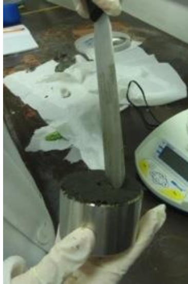
FIGURE C.7. THE SECTION OF SLUDGE THAT THE CONE PENETRATED IS REMOVED FROM THE CUP TO BE TESTED FOR MOISTURE CONTENT.
