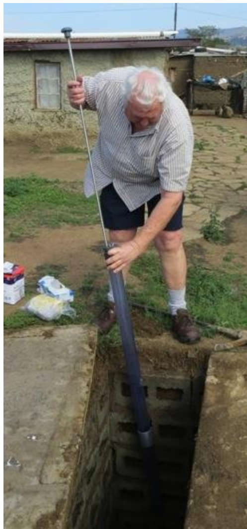
FIGURE H.1. ORIGINAL SAMPLING TUBE WHICH WAS UNSUCCESSFUL
