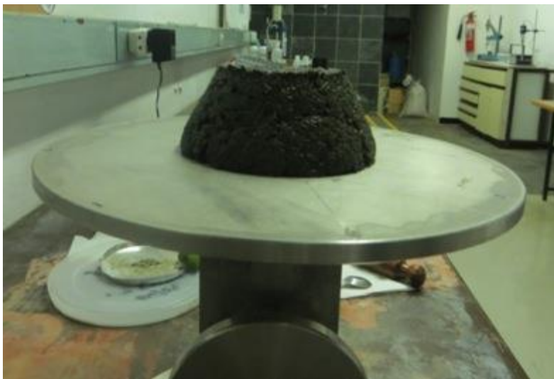
FIGURE B.8. SLUDGE AFTER DROPS HAVE BEEN APPLIED, THIS IS A DRY SAMPLE AND HAS NOT CHANGED MUCH FROM ITS' ORIGINAL POSITION
