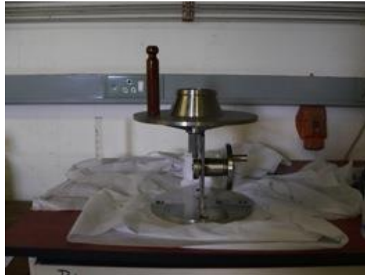
FIGURE B.1. FLOW TABLE APPARATUS, INCLUDING FLOW TABLE, WOODEN TAMPER AND METAL MOULD
