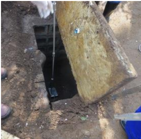
FIGURE H.8. BUCKET SAMPLER IN PIT TO RETRIEVE A SAMPLE. AGAIN, THE LONG HANDLE COMPRISES OF SEVERAL SHORTER PIECES THAT ARE FIT TOGETHER TO THE DESIRED LENGTH
