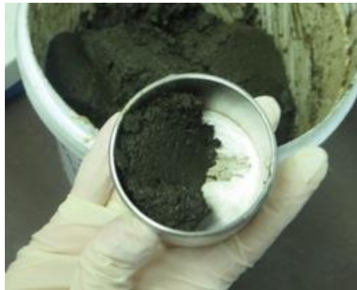
FIGURE C.2. SAMPLE CUP BEING FILLED UP, PRESSING SLUDGE TO THE SIDES TO ENSURE NOT AIR POCKETS ARE CREATED
