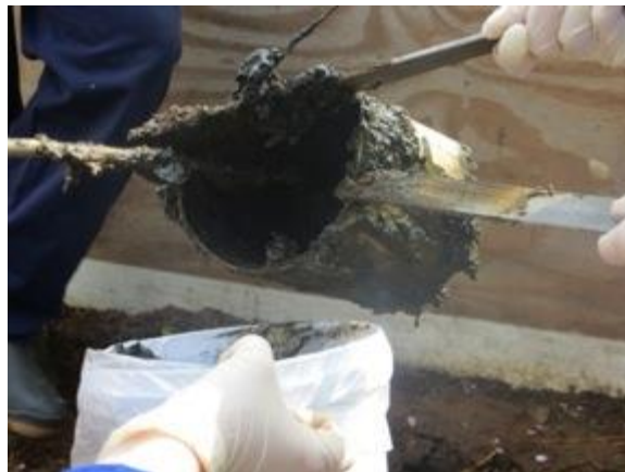
FIGURE H.9. ATTACHABLE HANDLES USED TO EASILY TIP BUCKET TO EMPTY CONTENTS INTO THE STORAGE CONTAINER. A SLIT IS PLACED AT THE END OF ATTACHABLE HANDLE SO IT CAN BE USED TO GRIP THE RIM OF THE BUCKET AS WELL
