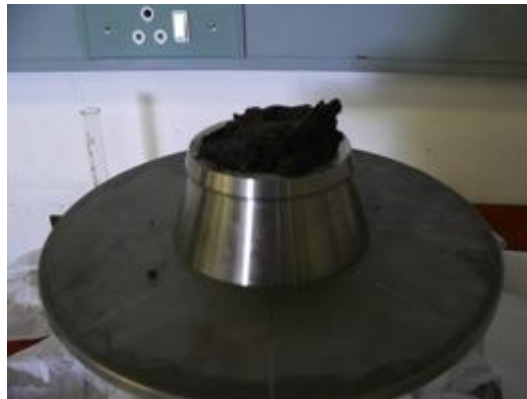
FIGURE B.2. FLOW TABLE MOULD FILLED WITH SLUDGE
