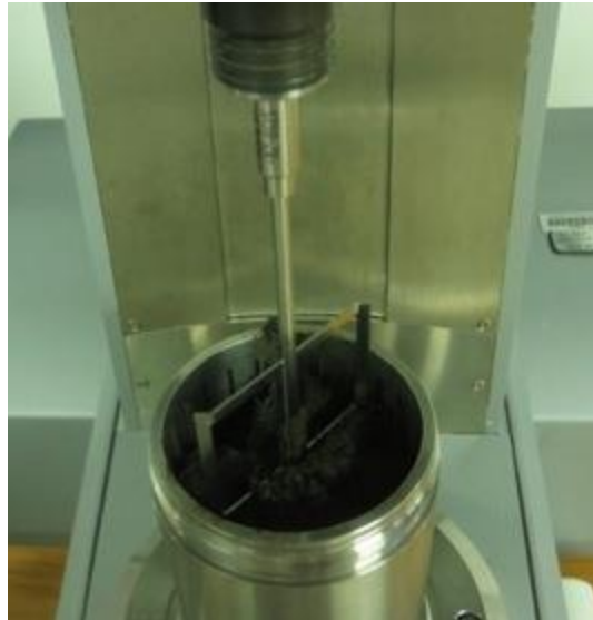
FIGURE D.3. THE VANE IS ATTACHED AND THE TEST IS STARTED VIA THE COMPUTER
