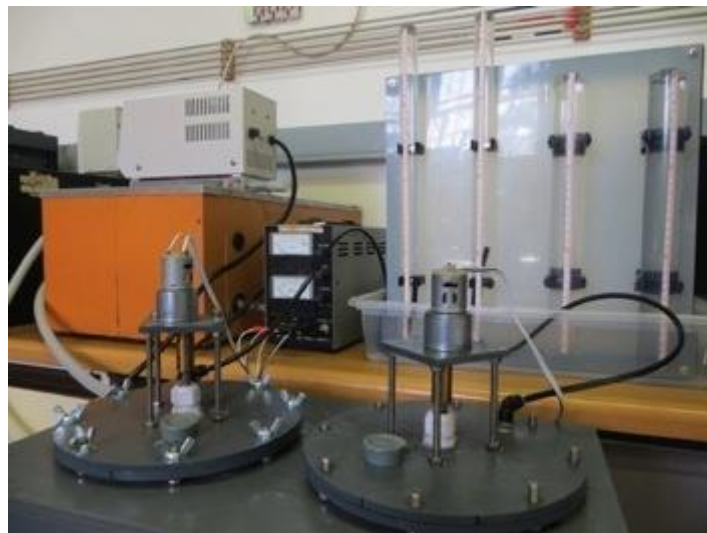
FIGURE E.4. VIEW OF THE LID OF THE TANKS AND THE MOTORS THAT POWER THE STIRRERS
