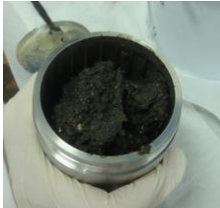
FIGURE D.1. SLUDGE SAMPLE PLACED WITHIN THE CYLINDER WHICH ATTACHES TO THE RHEOMETER MACHINE
