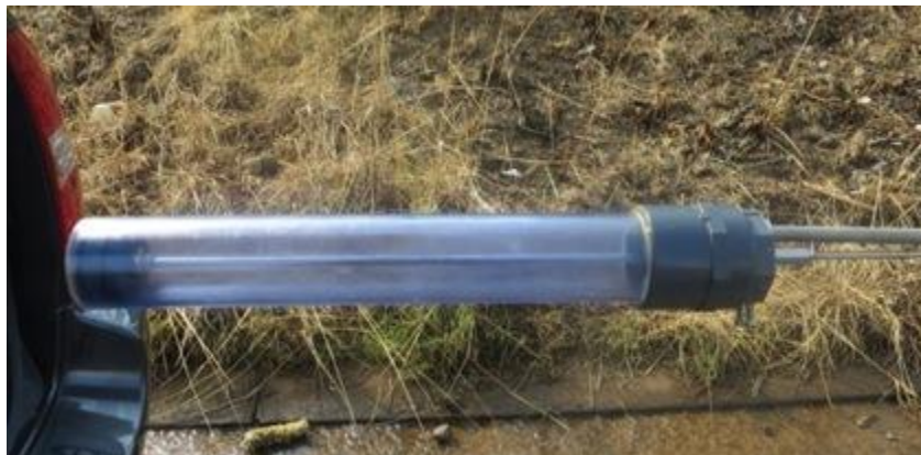
FIGURE H.3. SAMPLING TUBE DEVELOPED TO TAKE CORE SAMPLE OF DRIER SLUDGE
