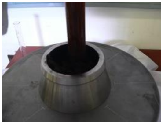
FIGURE B.3. TAMPER BEING USED TO COMPACT SLUDGE INTO THE MOULD
