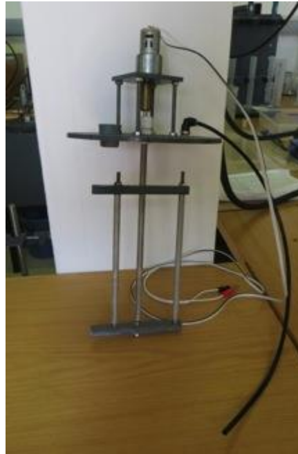
FIGURE E.3. THE STIRRER AND LID, WHICH IS SCREWED ONTO THE TANK, ON TOP OF WHICH IS THE MOTOR TO POWER THE STIRRER AND THE OUTLET PIPE THAT DIRECTS THE GAS INTO THE CYLINDERS
