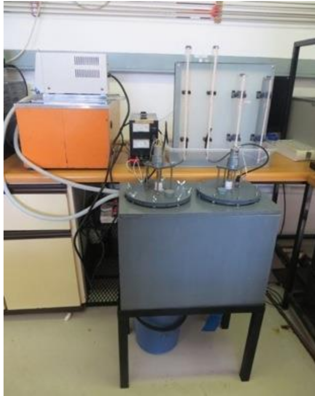
FIGURE E.1. CSTR SETUP, CONSISTING OF TWO TANKS HELD IN THE INSULATED GREY BOX, THE ORANGE WATER BATH AT 35°C ON THE LEFT AND THE INVERTED CYLINDERS ON THE RIGHT TO MEASURE THE GAS PRODUCTION
