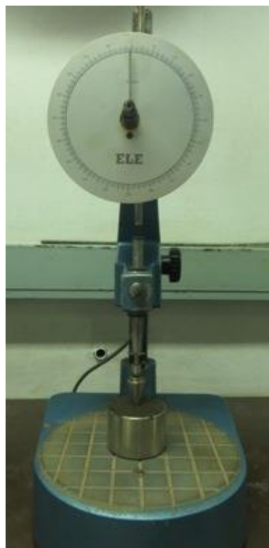
FIGURE C.6. THE DIAL IS TURNED UNTIL THE ROD MEETS THE BAR CONNECTED TO THE CONE AND THE READING TAKEN IS THE PENETRATION
