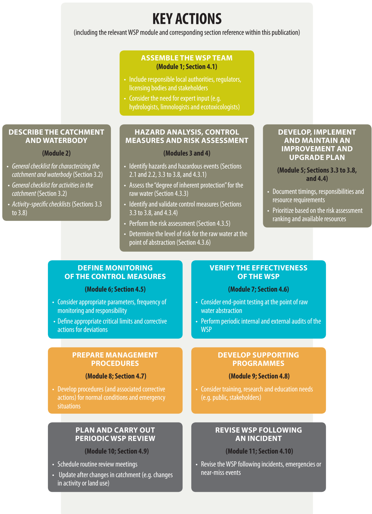
Figure 3 Summary graphic of catchment-related actions (modules) within the WSP framework (after Bartram et al. 2009) and the corresponding section in this publication
