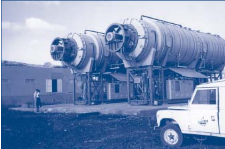
Fig. 18.6. Mechanical vapour compression (MVC) plant in Praia, Cape Verde (capacity: 2 \times 1250 \text{ m}^3/\text{day} ) (photograph by Jan C. Schippers)
