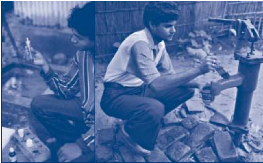
Fig. 23.2. Testing of tubewell water by a field test kit (left) and a contaminated handpump being painted red indicating that it should not to be used for drinking and cooking (right).
