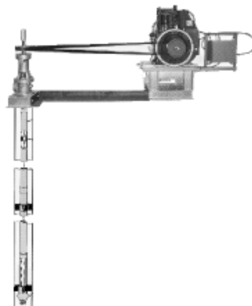
Figure 32 Diesel driven pump
