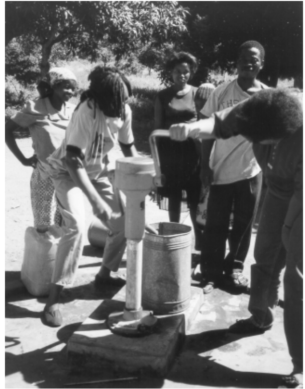
Figure 26 Progressive Cavity Deep Well Pump
