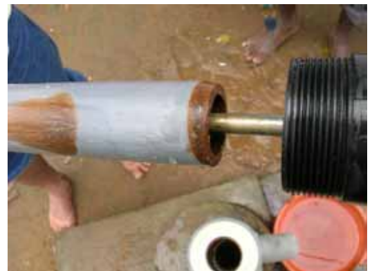
Andranofotsy AB 07/06, abrasion on pumprod pipe end
