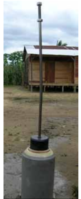
Andranofotsy AB 29, bent pumprod
