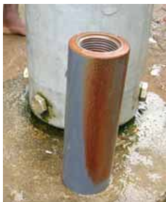
Andranofotsy AB 07/06, abrasion on pumprod and plunger
