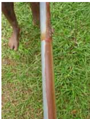
Andranofotsy AB 07/06, abrasion on pumprod and plunger
