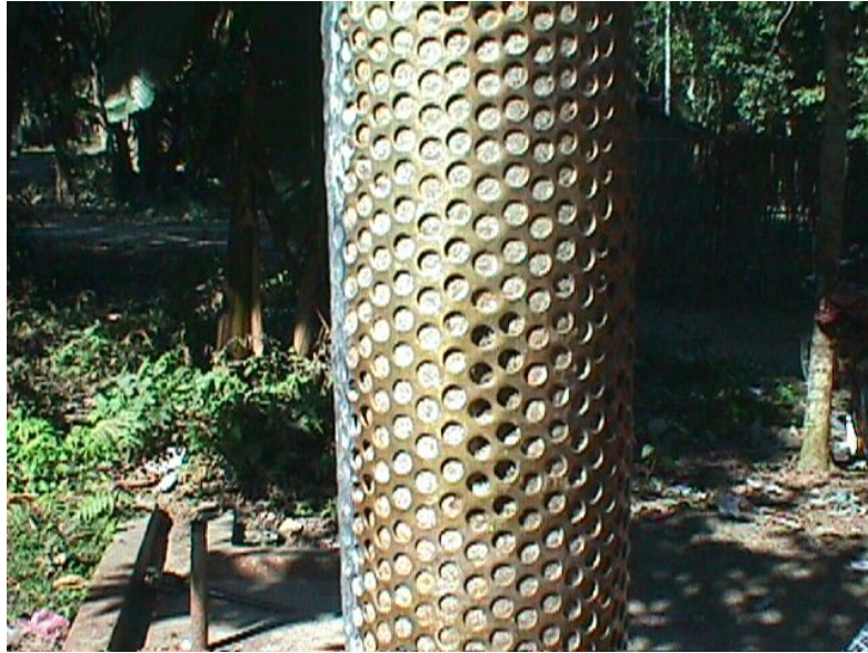
Figure 15: Screen formed from Galvanised Pipe with Pressed out Holes Covered in Brass Sheet
