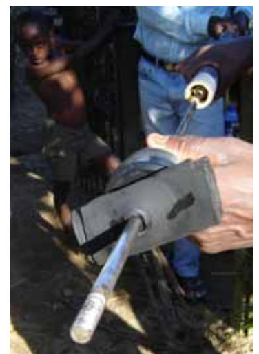
Nandrahanana N 01, pumprod broken, (see short thread)
