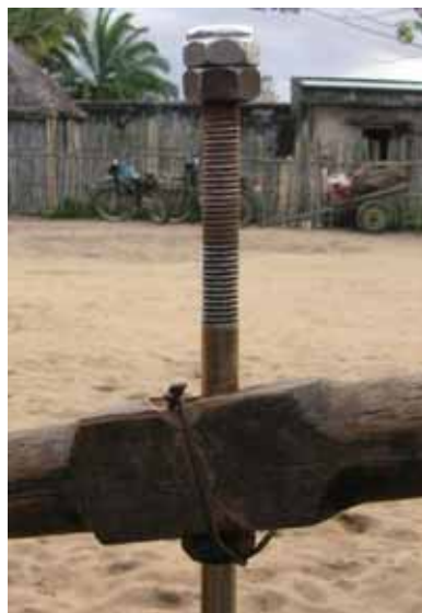
Maroantsetra, outside prison thread of lower nut worn (see position)
