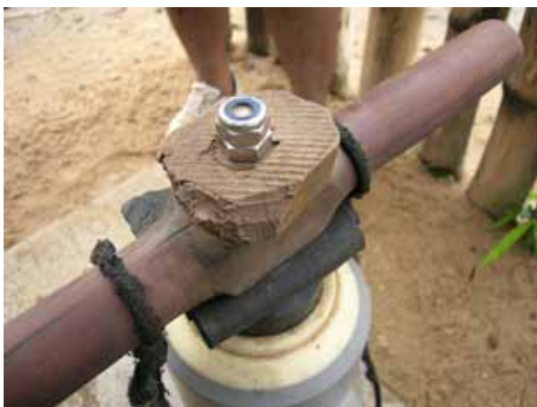
Mahalevona MV 18, clever handle repair
