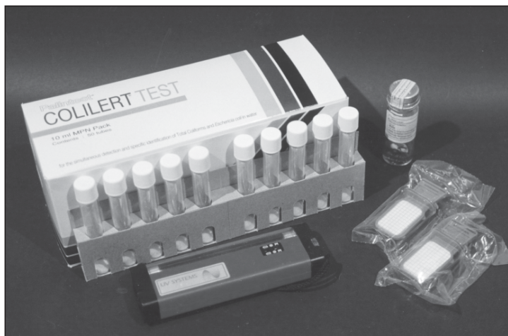
Colilert test, H 2 S strip and dipslides
