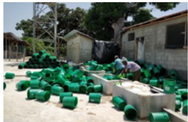
Figure 21. SOIL composting site. Transfer of container content to composting bins and disinfection of cleaned buckets with chlorine solution. Photo credit: SOIL (left) and Lars Schoebitz (right)
