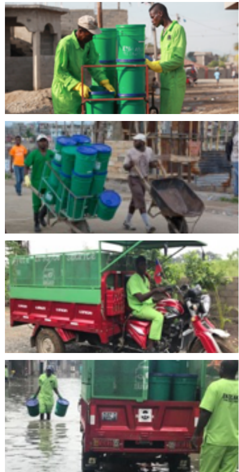
Figure 17. SOIL collection of containers used inside CBS toilets. Depending on the density of the neighbourhood, appropriate modes of transport are developed, such as modified wheelbarrows and three-wheeled motorcycles. Photo credit: SOIL
