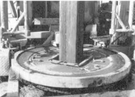
Figure 10.20. A rotary table rotates the kelly, which is connected to the top of the drill string. The kelly can be square, hexagonal, or round with flutes cut into the outer wall. ( Huron Drilling )
