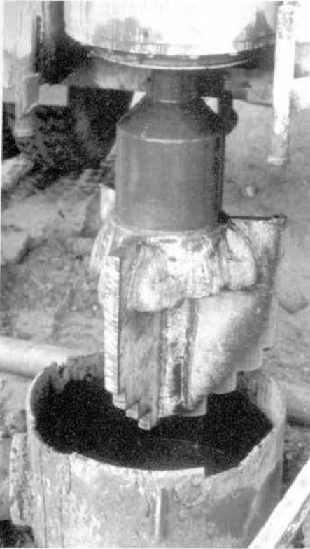
Figure 10.13. Drag bits are used in rotary drilling for fast penetration in unconsolidated or semiconsolidated sediments.
