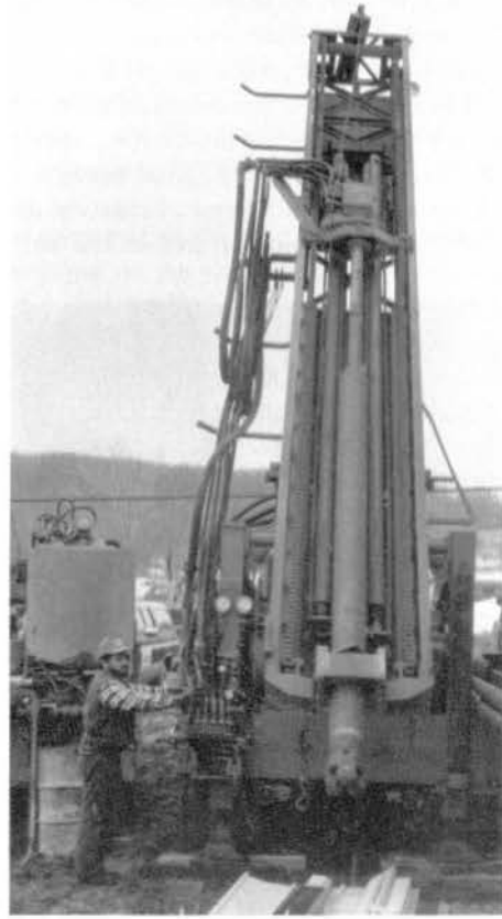
Figure 10.22. On some direct rotary rigs, a top-head drive is used to rotate the drill string. The amount of torque delivered to the bit by a top-head drive is usually somewhat less than that produced by a table drive, but the rod-handling speed is exceptionally good. (Olson Brothers Well Drilling)
