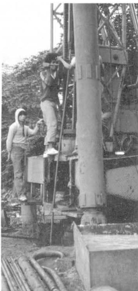
Figure 10.18. Stabilizers mounted just above the bit in the drill string are important in maintaining a straight borehole. Flat-bar steel plates welded to the stabilizer help maintain borehole diameter and provide channels for the passage of drilling fluid. (Hydro Drillers)
