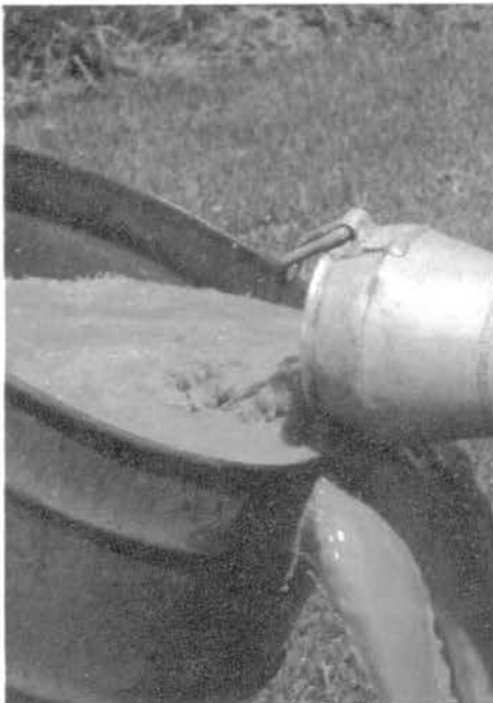
Figure 15.25. The concentration of suspended sediment can be estimated by collecting water and sediment in a large container. (Olson Bros. Well Drilling Company, Inc.)
