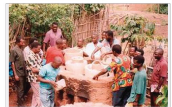
This outdoor kiln is suitable for the firing of the components of the stoves
