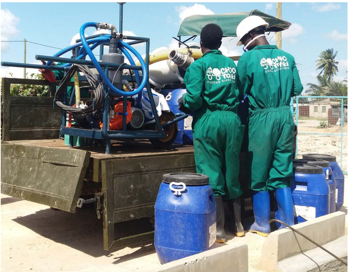
Figure 9 Small-scale E&T equipment: eVac and motorised tricycle at Mburahati-Ubungo FSTP
