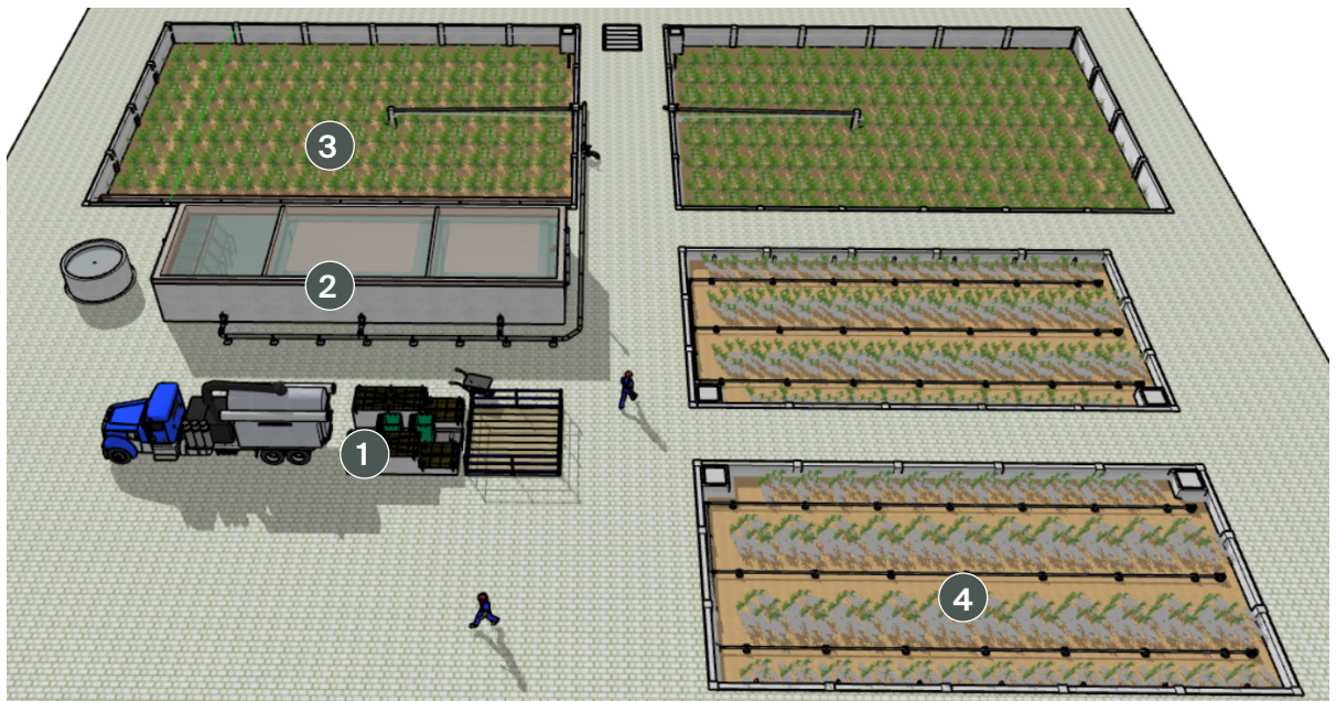
Receiving Station (1), Anaerobic Stabilization (2), optional with biogas, Planted Drying Beds (3), Vertical Flow Constructed Wetland (4)
