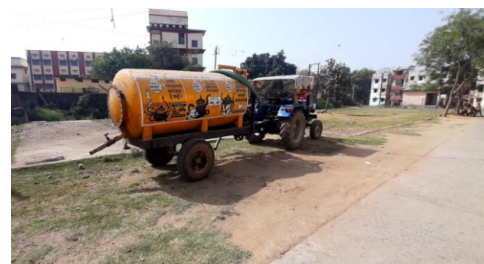
Figure 7: Transportation of Faecal Sludge through Vacuum Tanker (CSE/Manish Mishra, 2021).
