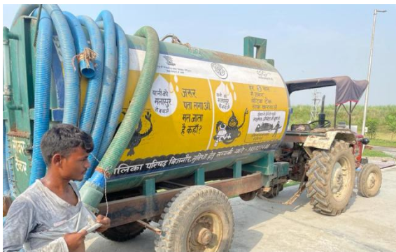
Figure 8: Government desludging tractor-mounted machine for decanting in broader lanes (Source: Harsh/CSE/2021).
