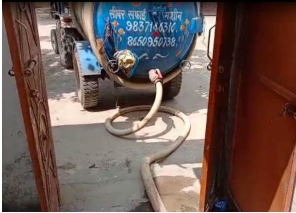
Figure 10: Emptying being done by mechanical means (Aamir/CSE/2021).
