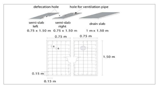
Figure 13.6: Reinforcement for a two-part symmetrical slab.
