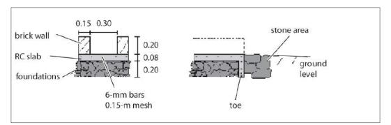
Figure 10.15: Drainage channel (A) and toe (B).
