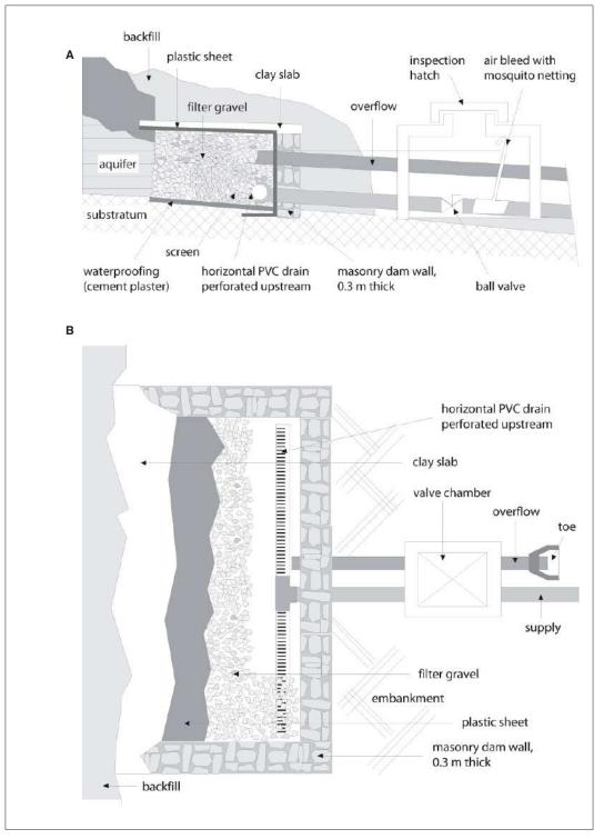
Figure 10.2: Infiltration gallery. A: section. B: plan.
