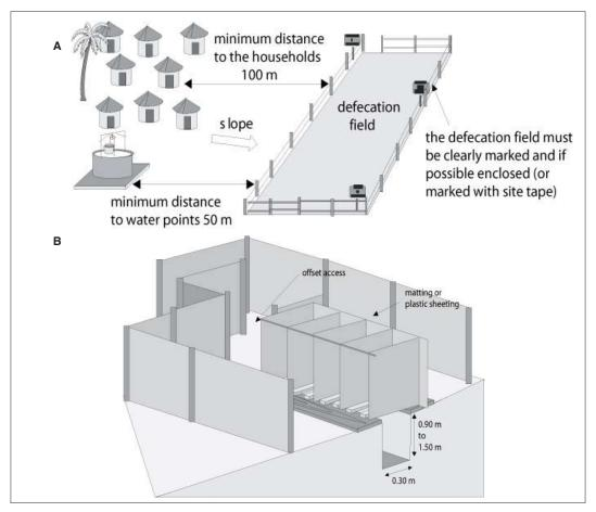
Figure: 13.22: Defecation management in the first (acute) phase of an emergency. A: defecation field. B: defecation trench.
