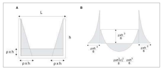
Figure 36: Rectangular tank subject to water pressure.
