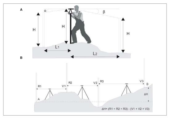
Figure 11.4: Topographic survey. A: with Abney level or clinometer. B: with dumpy level.
