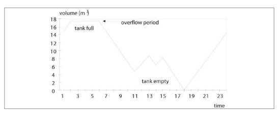
Fig 10.6: Representation of volume of water in a tank over one day.
