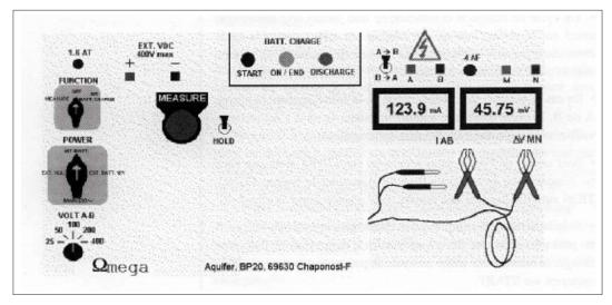
Figure 1: Front of the  $\Omega$ mega resistivity meter.
