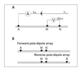
infinite distance electrode (Figure 5.18). In a onedimensional medium the two soundings are identical; any difference means that the medium is heterogeneous and one-dimensional soundings are inadequate (see Box 5.2).
