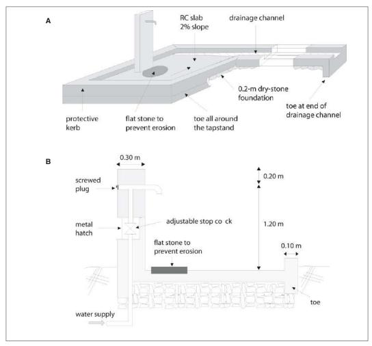
Figure 11.33: Reinforced-concrete tapstand with one tap. A: general view. B: section.
