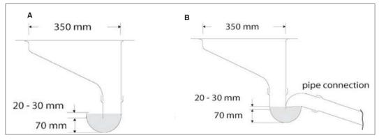
Figure 13.10: Water seal. A: placed over the pit. B: with an off-set pit.
