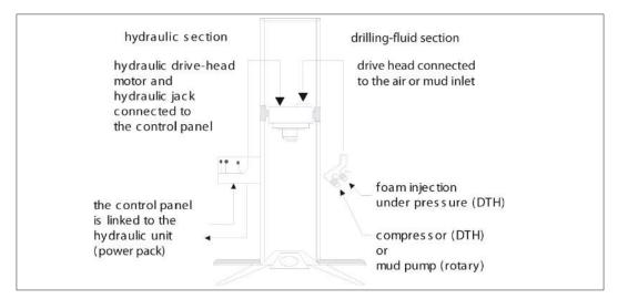
Figure 8.7: The ACF-PAT 301 drilling rig – working principle.
