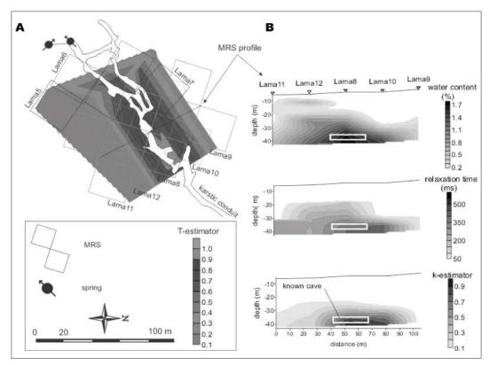
Figure 5.86: MRS Karst localisation. A: conduit mapping using T-estimator. B: cross-section using k-estimator.
