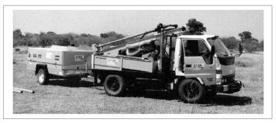
Figure 8: ACF-PAT 401. Rig on a Dyna truck.
