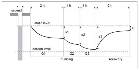
Figure 6.15: Well test in connected steps.
