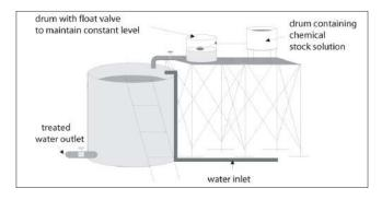
Figure 12.9: Addition of chemical at a constant rate.
