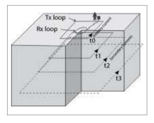
sured at the surface. As the currents penetrate more deeply with time, measurement of the secondary field at the surface at different times gives information from different depths. The receptor (Rx) is usually a pre-wound multiple loop, a simple loop of cable placed on the ground that could be the same loop as that used previously as Tx.
