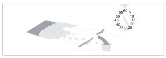
Figure 3.3: Direct flow measurement.
