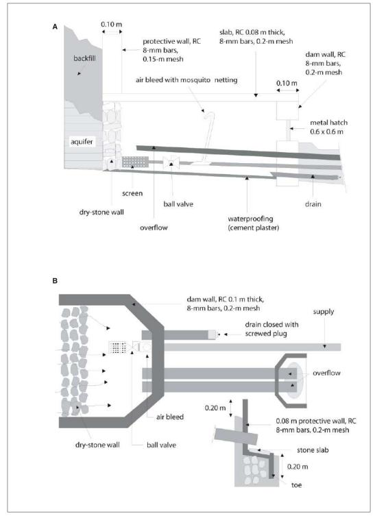
Figure 10.1: Spring box in reinforced concrete. A: section. B: plan.
