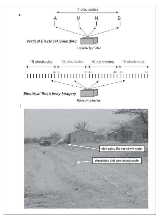
Figure 5.30: ERI measurement array.
