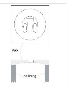
Figure 13.8: Rectangular dome-shaped slab.
