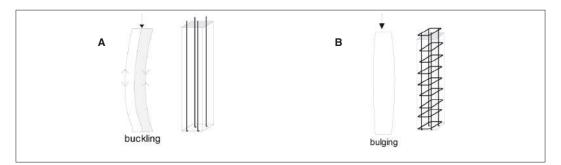
Figure 34: Reinforcement of a pillar to reabsorb all the stresses acting on the structure.. A: to avoid buckling, which deforms the pillar and leads to tensile strain, longitudinal reinforcement is used. B: bulging of a section is restricted by the placing of transverse frames, which also facilitate the location of longitudinal bars.
