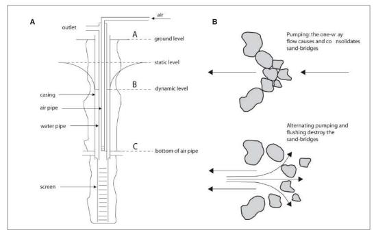
Figure 8.25: Air-lift. A: design. B: sand-bridge destruction.
