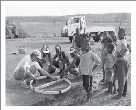
**Figure 5.57: Setting up a TDEM measurement (Mozambique, 2000).**
