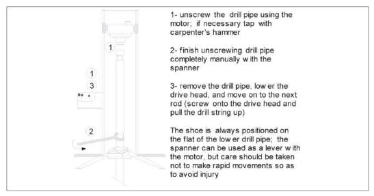
Figure 8.19: Removing a drill pipe.
