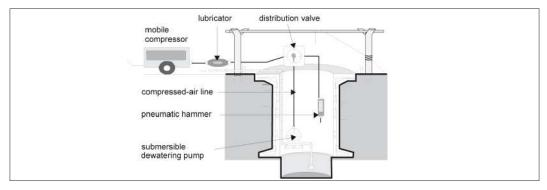
Figure 9.18: Using a pneumatic pump and a pneumatic hammer in well digging.
