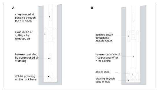
Figure 8.2: Working principle of DTH hammer drilling.
