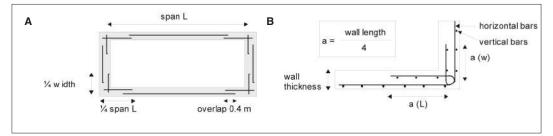
Figure 19: Reinforcement for a rectangular tank.
