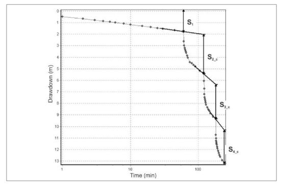
Figure 6.17: Graphical estimation of the corrected drawdown s<sub>i C</sub>, borehole 204.
