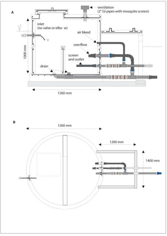
Figure 11.36: Header tank. A: section. B: plan.
