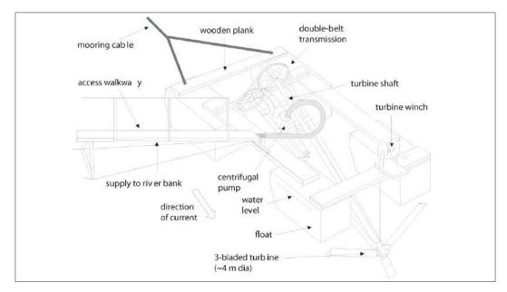
Figure 9.22: Garman pump installed on a raft.
