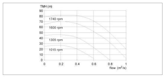
Figure 9.7: Characteristic curves for a centrifugal pump as a function of rotational speed.
