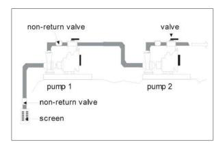
Figure 9.8: Mounting two identical pumps in series.
