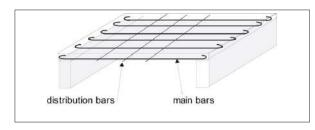
Figure 33: Reinforcement of a full slab supported on two walls.
