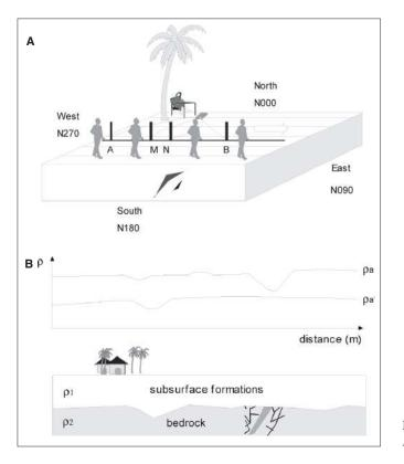
Figure 5.28: Resistivity profiling. A: setting up. B: example.
