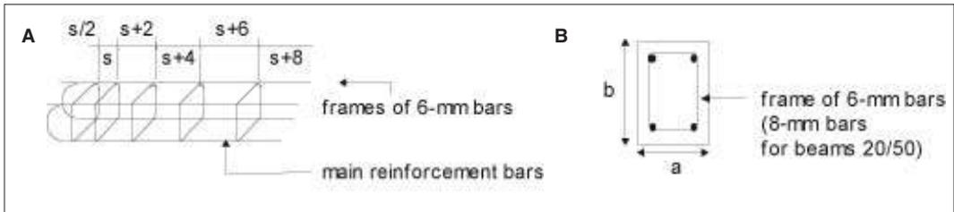
**Figure 8: Reinforcement mesh (A) and normal dimensions (B) for a beam.**
