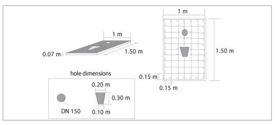
Figure 13.5: Reinforcement for a single slab.
