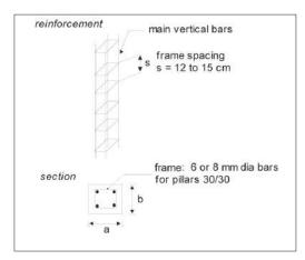
Figure 7: Reinforcement for a pillar.
