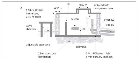
Figure 11.18: Masonry break-pressure tank. A: section.
