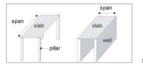
Figure 6: Span of a slab.
