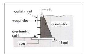
Figure 41: Standard configuration of reinforcedconcrete retaining walls.
