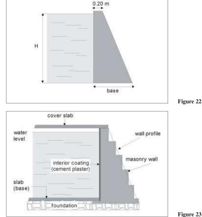
Figure 22: Retaining wall.
