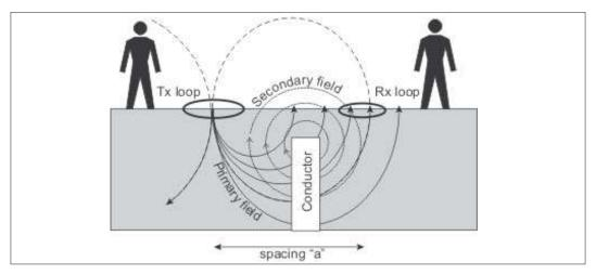
Figure 5.40: Slingram configuration (VD), EM 34.
