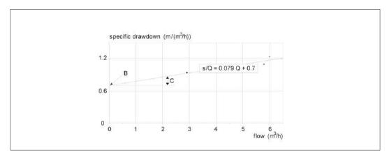
Figure 6.7: Calculation of head losses. Well test: borehole F1 – Estimation of head-losses using Jacob's method. Linear head-losses: B = 0.7 m/(m<sup>3</sup>/h). Quadratic head-losses: C = 7.9  $10^{-2}$  m/(m<sup>3</sup>/h)<sup>2</sup>.
