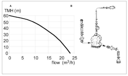
Figure 9.19: Membrane dewatering pump.
