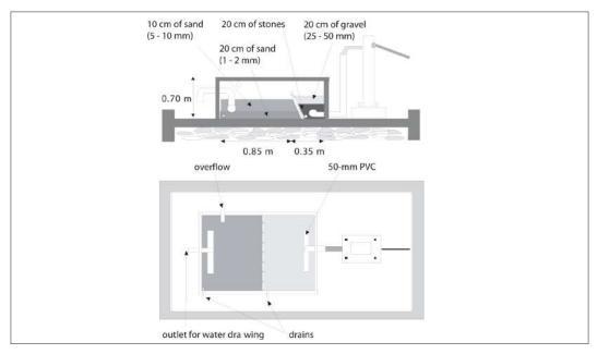
Figure 12.6: Removal of iron by aeration and filtration.
