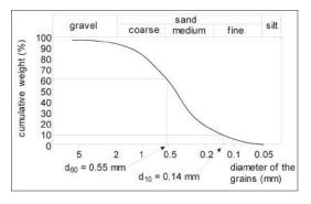
Particle-size analysis is based on a sample of the formation being studied. By successive screening, the various sizes of particle are separated and then weighed. The results are then represented in a standard curve (Figure 1), plotting the particle size in mm logarithmically on the horizontal axis and the percentage cumulative weight of successive screenings on the vertical axis.
