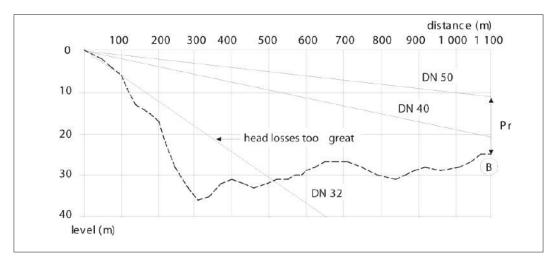
Figure 11.13: Head losses for different pipe diameters for the first part of the Aloua system.
