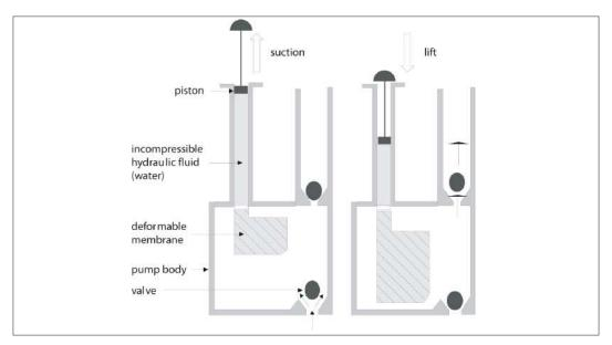
Figure 9.33: Working principle of Vergnet hydropump.
