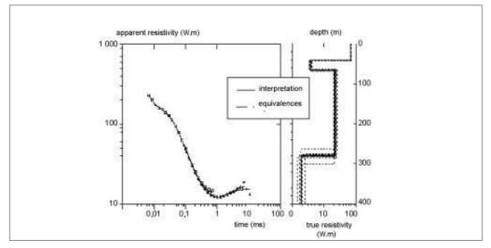
Figure 5.45: Example of TDEM sounding (ACF, Cambodia, 1998).
