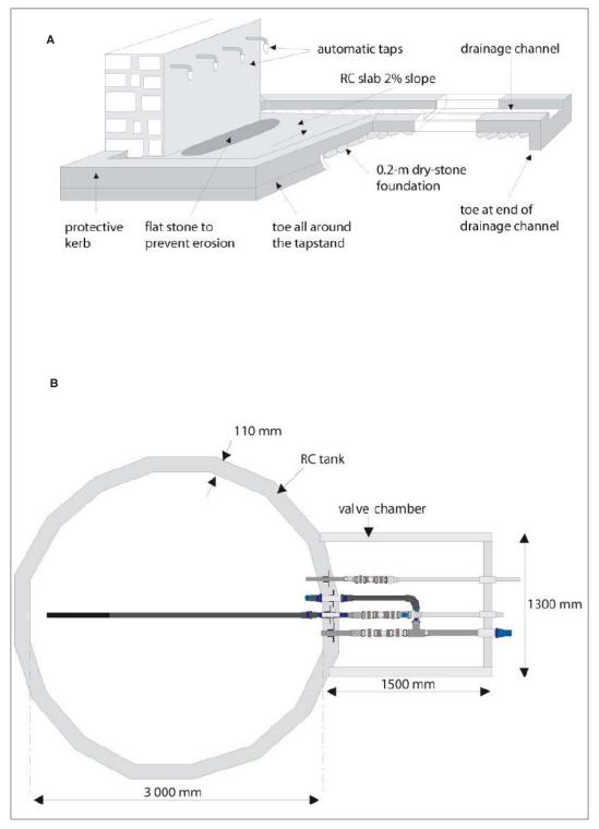
Figure 11.35: Reinforced concrete tank (ACF, Laos, 1998). A: section. B: plan.
