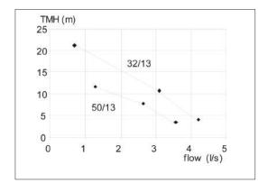
Figure 9.23: Characteristic curves for Garman 32/13 and 50/13 pumps. Current speed: 0.85 – 0.9 m/s; large blades (ACF, Sudan, 1996). These two pumps mounted in series on the Nile at Juba produced around 2 l/s for a TMH of 25 m.
