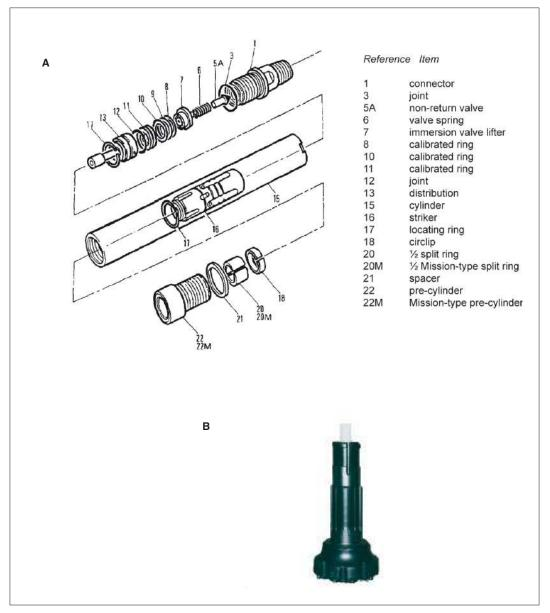
Figure 12: Down-the-hole hammer. A: DTH-hammer parts list. B: drilling bit.
