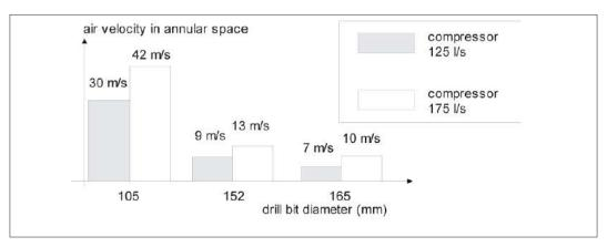
Figure 8.5: Air velocity as a function of compressor flow and drill bit diameter.
