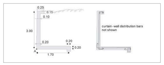
Figure 14: Dimensions and arrangement of reinforcement of a reinforced-concrete retaining wall 3 m high.
