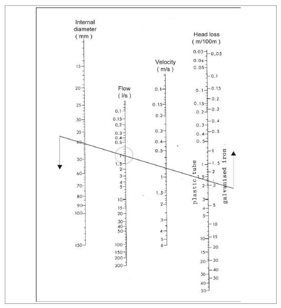
Figure 11.10: Design chart for calculating linear head-losses.
