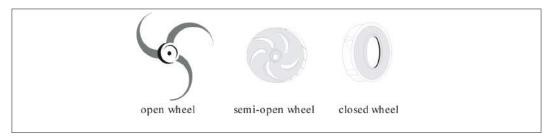
Figure 9.3: Rotor designs in centrifugal pumps.
