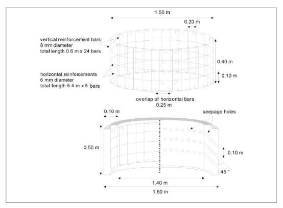
Figure 7.11: Reinforcement of perforated rings.
