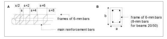
Figure 8: Reinforcement mesh (A) and normal dimensions (B) for a beam.
