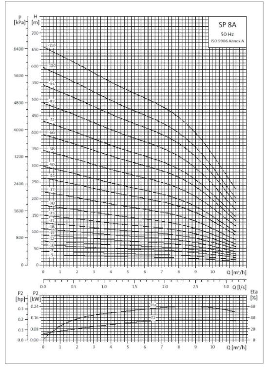
Figure 9.5: Characteristic curve for the Grundfos SP8A range of pumps, and efficiency curves where Q = flow, H = TMH, and  $\eta =$  efficiency.
