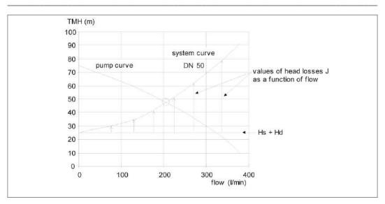
Figure 9.6: Working point (TEF2-50 pump in pipe system).
