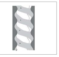
Figure 9.35: Helical rotor of the Monolift pump.
