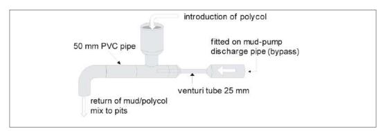
Figure 8.14: Venturi mixer made from PVC fittings.
