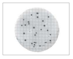
The culture medium used is the ready-to-use Millipore MFC (membrane faecal coliform) broth, which develops a specific colour with faecal coliforms. ACF also uses disposable plastic sachets for sterile water sampling.
