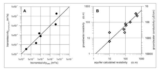
Figure 5.74: MRS hydraulic characterisation. A: local aquifer transmissivity B: groundwater electrical conductivity.
