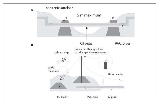
Figure 11.28: Crossing over ravines or rivers. A: use of a GI sleeve. B: suspended pipe. The following aspects should be given special attention:
