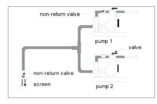
Figure 9.10: Mounting two pumps in parallel.
