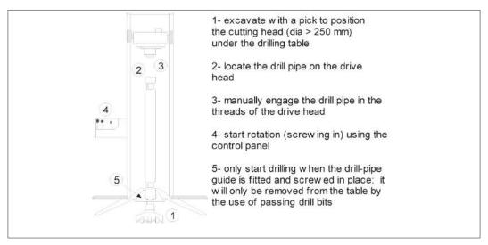
Figure 8.16: Fitting the first drill-pipe.
