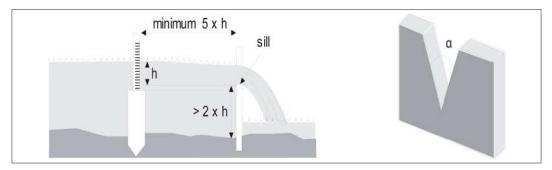
Figure 3.4: Thin-plate weir.
