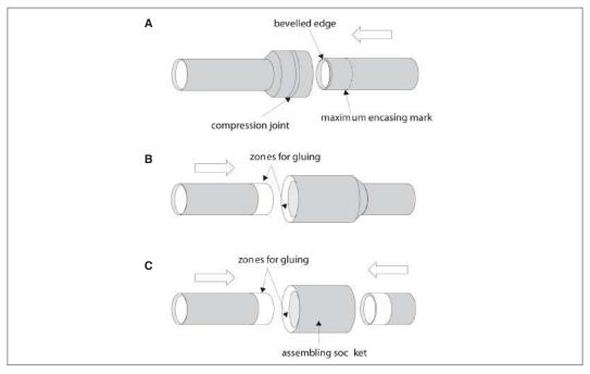
Figure 11.22: PVC pipe joints. A: rubber joint. B: glued joint. C: socket joint.
