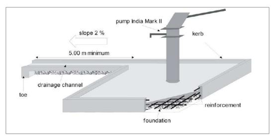
Figure 8.26: Borehole surface works (ACF, Kampala, Uganda, 1996).
