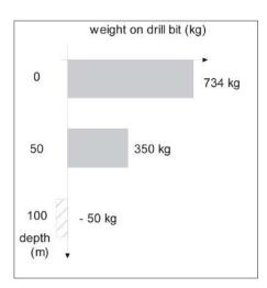
times low, particularly with lightweight rigs. On the other hand, at great depths, the drill string must be supported so as not to apply excessive pressure on the drill bit (Figure 8.4). The pressure to be applied on a tricone bit (rotary) is much higher than that applied on a DTH bit, but rotational speed is reduced (Box 8.1).
