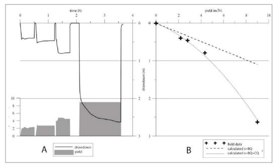
Figure 5.71: Pumping test, ACPI school. A: field measurements. B: head-loss calculation.
