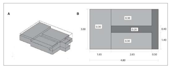
Figure 10.9: Foundations of tapstand and laundry area. A: perspective view. B: plan.
