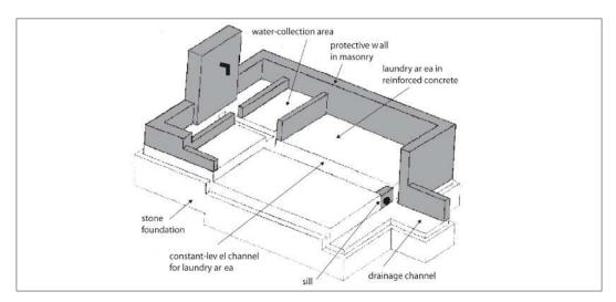
Figure 10.4: Examples of water points. B: water point with laundry area (ACF, Ethiopia, 1993).
