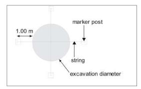
Figure 7.4: Marking the axis of excavation.
