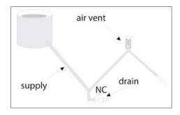
Figure 11.32: Drain and air vent.
