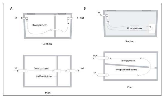
Figure 13.13: Septic tank flow pattern (adapted from Crites & Tchobanoglous, 1998). A: interior baffle placed across tank. B: interior baffle placed longitudinally.
