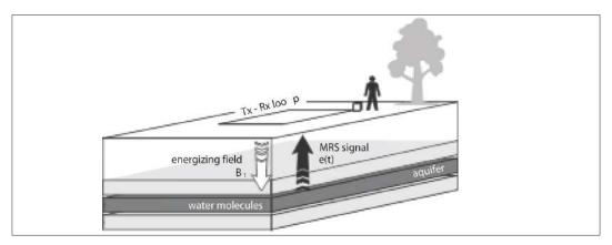
Figure 5.48: Schematic diagram of MRS measurement array.
