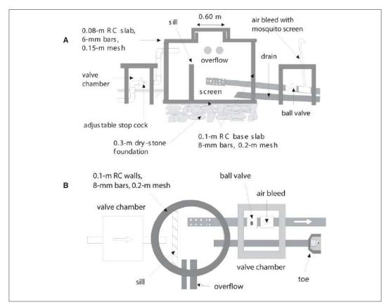
Figure 11.19: Reinforced concrete break-pressure tank. A: section. B: plan.
