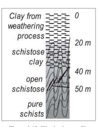
Figure 3.14: Weathering profile of granites.
