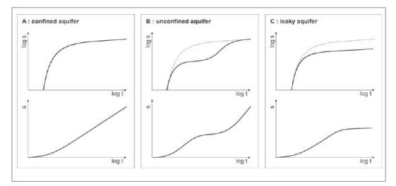
Figure 6.1: Theoretical diagnostic graphs of aquifer type showing drawdown (s) against time (t). The dashed curves are those of the 'ideal confined aquifer' as represented on graph A (Kruseman & de Ridder, 2000).
