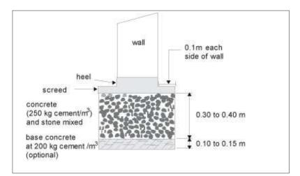
Figure 15: Section through a foundation.
