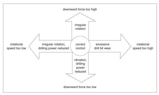
Figure 8.3: Control of downward force and rotation.
