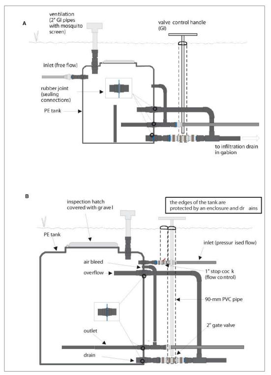
Figure 11.37: Polyethylene tank. A: header. B: tank.
