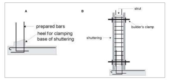
Figure 44: Shuttering for a pillar or curtain wall. A: awaiting shuttering and reinforcement. B: shuttering and reinforcement in place.
