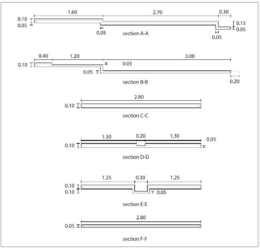
Figure 10.12: Sections of the slab.
