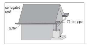
Figure 3.2: Harvesting of water from a roof.
