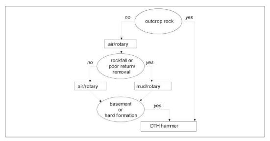
Figure 8.11: Flow chart for selection of drilling technique.
