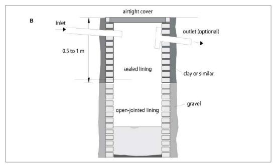
Figure 13.16: Soakaway pits. B: lined pit.
