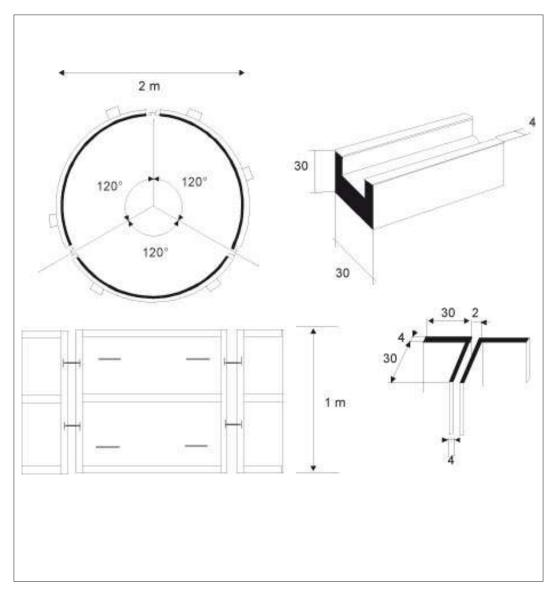
Figure 48: Shuttering for a headwall (2 m external diameter)
