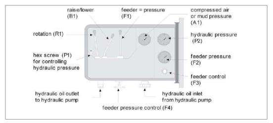
Figure 8.8: Control panel functions on the ACF-PAT 301 (1996 model).
