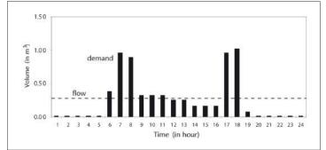
Figure 1: Comparison of hourly demand and spring flow. Spring flow (l/h) < hourly demand → storage is required (tank).
