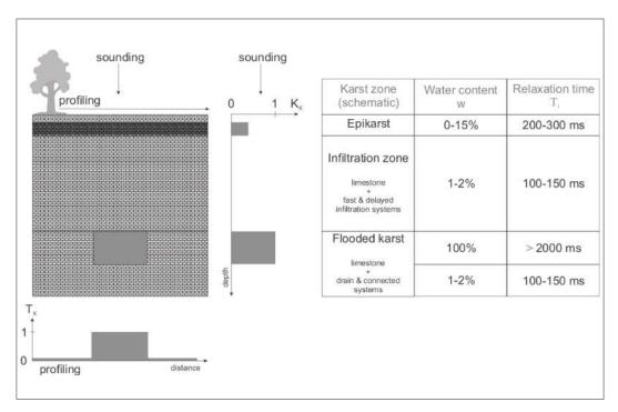
Figure 5.84: MRS estimators as tools to detect saturated karst structures.
