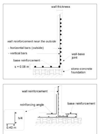
Figure 20: Wall reinforcement for a small rectangular tank: wall length less than 2 m, with overlap ('a' in Figure 19) 40 cm minimum.
