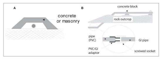
Figure 11.27: Passage above ground. A: masonry protection for pipe. B: use of GI pipe.
