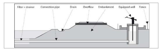
Figure 19.4: Well connected to pond.
