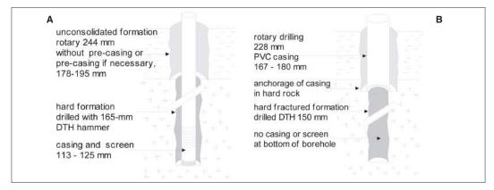
Figure 8.10: Mixed drilling using both rotary and DTH techniques. A: complete equipment. B: partial equipment for partly consolidated formations.
