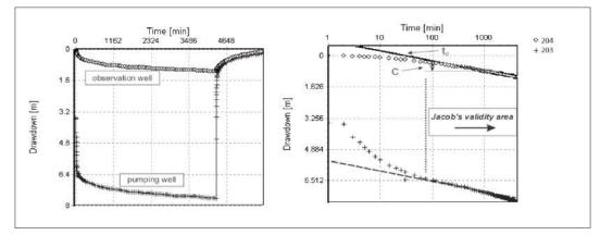
Figure 6.3: Aquifer-test interpretation using Jacob's method.
