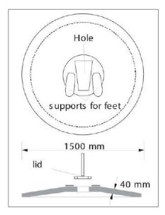
Figure 13.7: Round dome-shaped slab.
