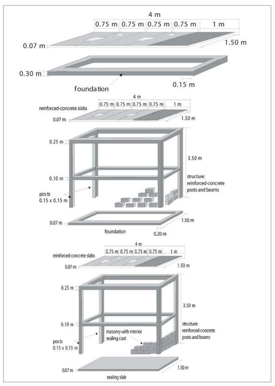
Figure 13.4: Pit and foundation of 2-station latrine.
