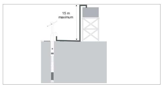
Figure 9.36: Pumping to a tank using a Monolift pump.
