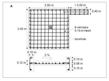
Figure 26: Reinforcement. A: slab.
