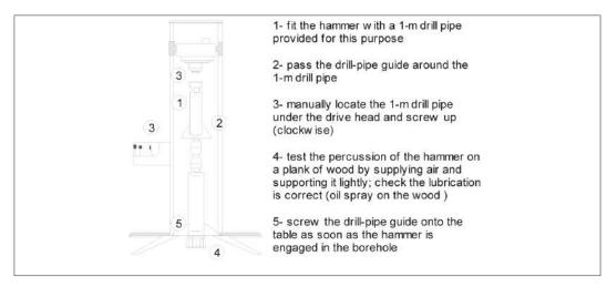
Figure 8.21: Fitting the hammer.
