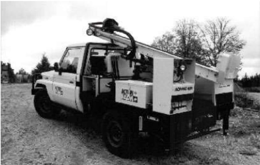
This rig is more powerful than the PAT 301, it is more easily manoeuvrable, and the set-up time is less. The vehicle can be set level immediately with the jacks. The rig can be used in rotary mode, and in DTH 5" mode (165 mm bit). The drilling depth is more than 100 m in sedimentary formations. ACF has used this rig in Angola (Dyna version), and Honduras (Land Cruiser version).
