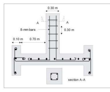
Figure 30: Reinforcement for tapstand and apron.
