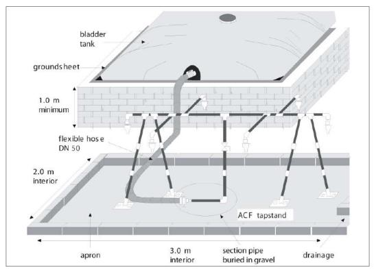
Figure 17.3: Flexible tank (bladder type) and tapstand.
