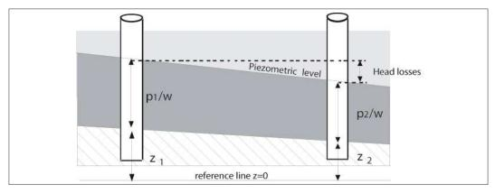
Figure 1: Flow in a porous environment.
