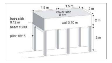
Figure 37: Elevated rectangular tank.
