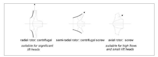
Figure 9.2: Rotor designs in turbopumps.
