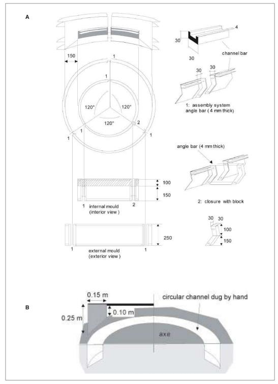
Figure 46: Shuttering for cutting ring. A: metal. B: mould made directly in the ground
