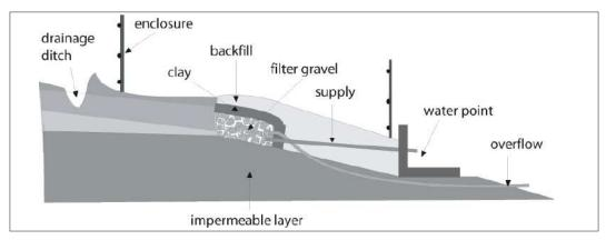
Figure 10.3: Infiltration gallery sealed with clay.
