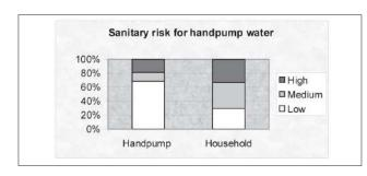
Figure 15.6: Sanitary risk for handpump water. The results of a study carried out in Myanmar show that water becomes contaminated between collection (at the handpump) and consumption (in the house). It suggests bad water-handling practices.
