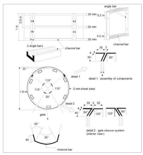
Figure 47: Sliding shuttering for a 1.8-m diameter well.
