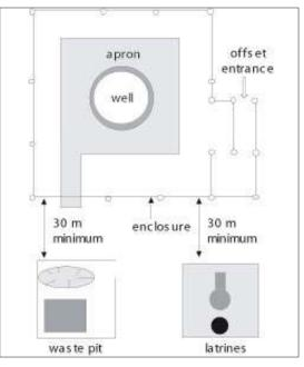
Figure 1: Protection zone of a well/borehole in a continuous environment.
