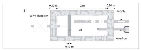
Figure 11.18: Masonry break-pressure tank. B: plan.
