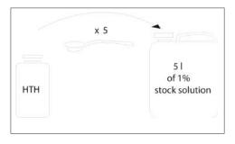
Figure 12.3: Preparation of stock solution of chlorine.
