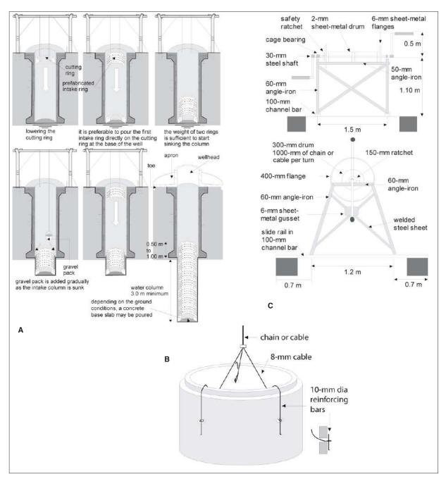
Figure 7.13: Sinking an independent intake.
