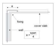
Figure 12: Reinforcement for a semi-fixed slab.
