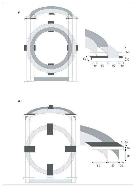
Figure 45: Metal shuttering for a concrete-ring mould. F: pedestal. G: cover.
