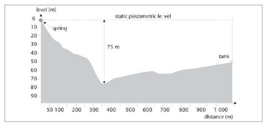
Figure 11.7: Static profile and pressure class of pipes.
