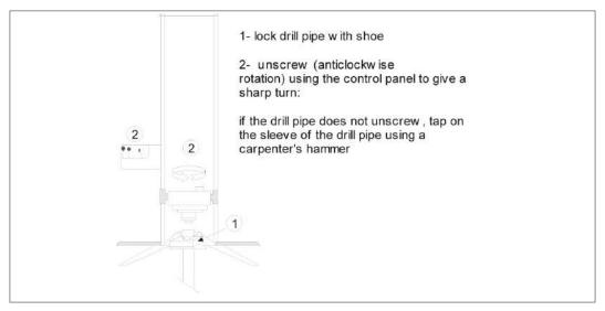
Figure 8.17: Unscrewing a drill pipe.
