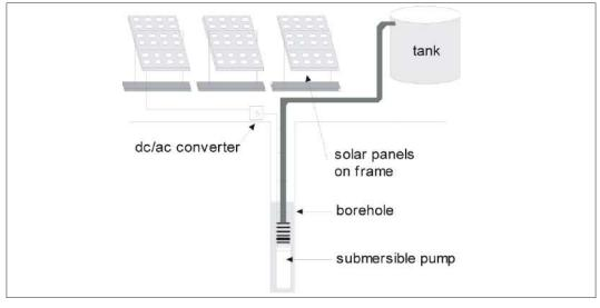
Figure 9.20: Supplying a pump using solar panels.
