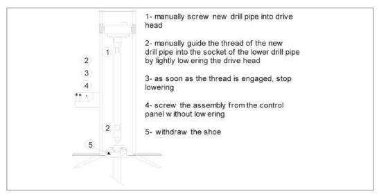
Figure 8.18: Locking drill pipes in suspension.
