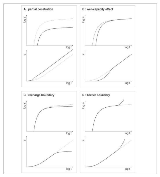
Figure 6.2: Theoretical diagnostic graphs of boundary conditions showing drawdown (s) against time (t). The dashed curve are those of the 'ideal confined aquifer' of Figure 6.1A (Kruseman & de Ridder, 2000).
