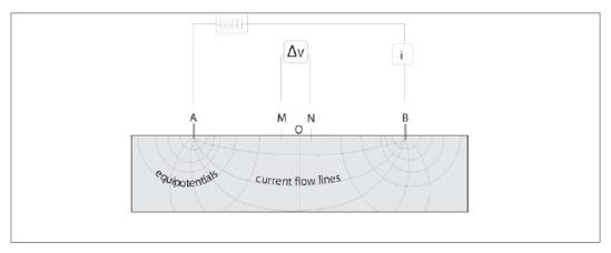
Figure 5.5: Principles of geophysical electrical measurements.
