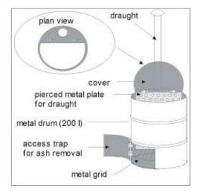
Figure 13.29: Simple incinerator.
