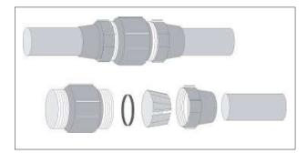
Figure 11.24: PE compression coupling.
