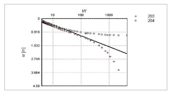
Figure 6.4: Aquifer-test interpretation using Theis's recovery method.
