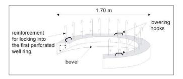
Figure 7.12: Cutting ring 1.4 / 1.6 m diameter.
