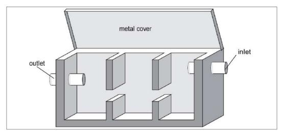
Figure 13.26: Grease trap, ACF Ingushetia 2003.
