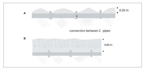
Figure 11.26: Backfilling the pipe trench. A: initial backfilling to test the pipes (pressurise system). B: final backfilling after pipe test.
