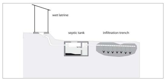
Figure 13.12: General view of wet toilet, septic tank and infiltration system.
