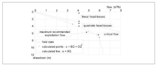
Figure 6.8: Well curve s = f(Q) of borehole F1.
