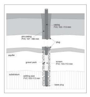
Figure 8.22: Borehole equipment (based on ACF, Uganda, 1997).
