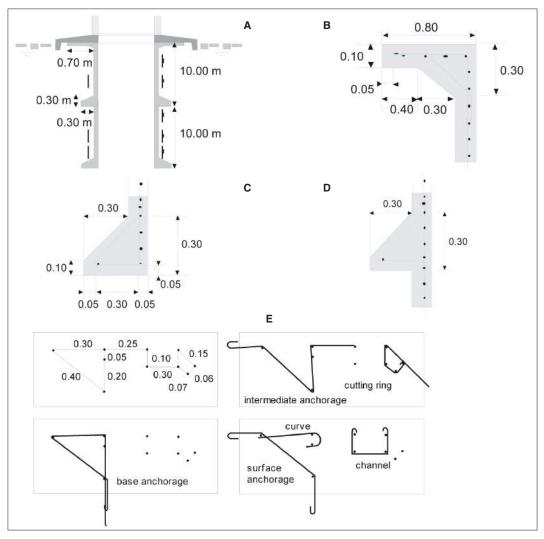
Figure 7.10: Reinforcement for lining anchorages.
