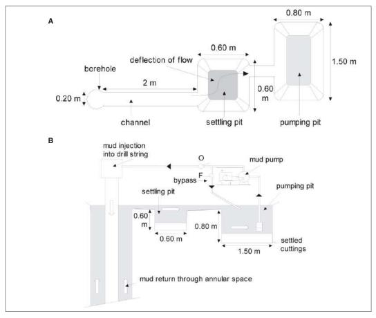
Figure 8.13: Mud circulation. A: plan view; B: section view.
