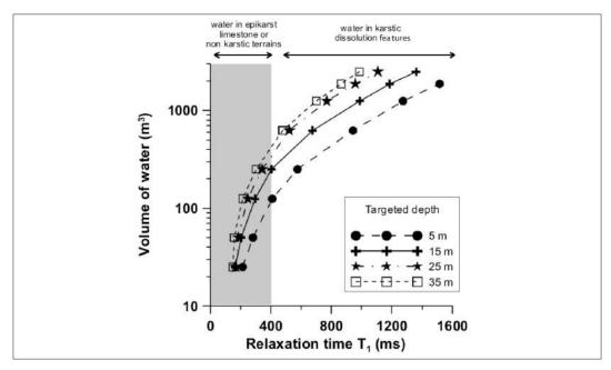
Figure 5.85: Required volume of free water (w=100% &  $T_1$ =1500 ms) for MRS measurements in a karstic environment (w=1% &  $T_1$ =150 ms).
