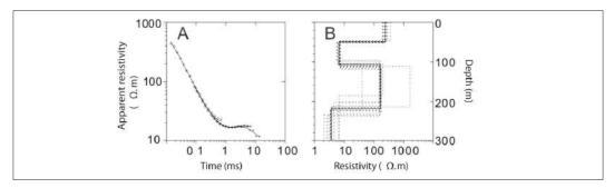
Figure 5.68: TDEM sounding, ACPI school. A: field data. B: inversion (equivalent models, best fit rms error = %).
