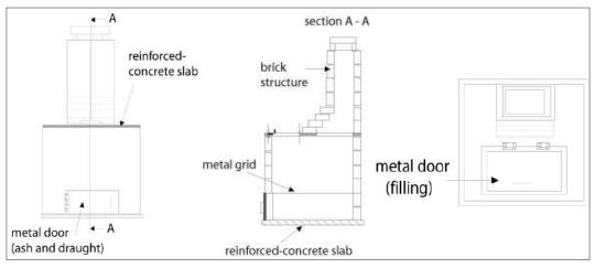
Figure 13.30: Brick-built incinerator.
