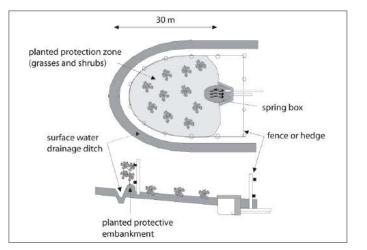
Figure 2: Protection zone of a spring.
