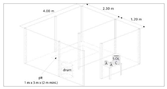
Figure 14.7: Example of excreta-disposal pit. Materials (without roof): posts, 27 m (8 x 8 cm), 36 m (4 x 8 cm). Plastic sheeting, 36 m<sup>2</sup>.
