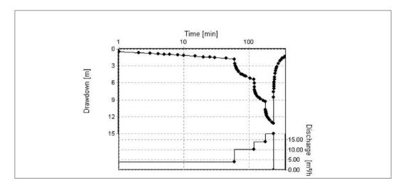
Figure 6.16: Four connected pumping steps, borehole 204.
