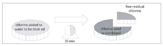
Figure 12.2: Chlorine in solution in water.
