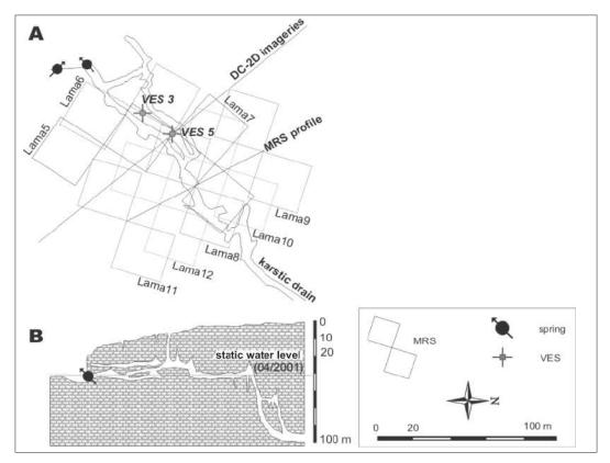
Figure 5.83: The known conduit system of Lamalou karst, and location of geophysical surveys. A: map. B: cross-section along the conduit.
