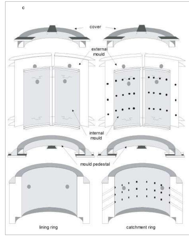
Figure 45: Metal shuttering for a concrete-ring mould. C: various parts of the mould. D: assembly details. E: numbering of various parts of the mould.
