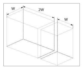
Figure 13.14: Design of the septic tank.
