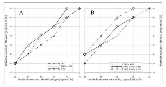
Figure 5.75: Cost-effectiveness boundaries of geophysical methods. A: use of a single method. B: joint use of methods.
