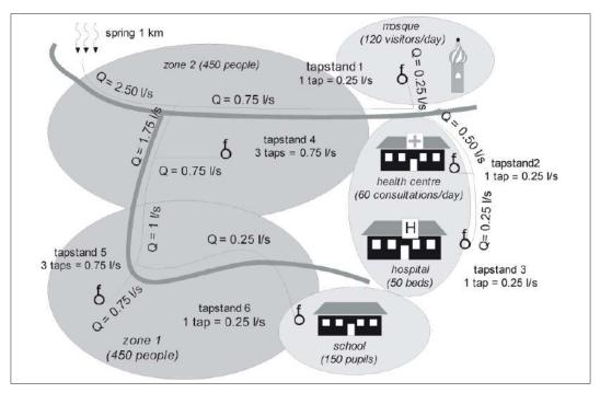
Figure 11.3: Marking out lines, flows and numbers of taps.
