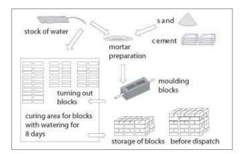
Figure 2: Plan of a mortar block workshop.
