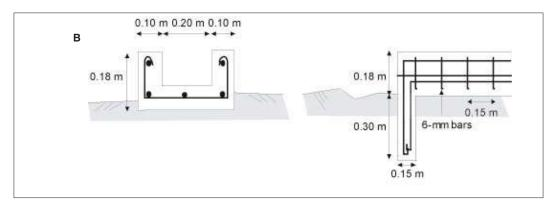
Figure 26: Reinforcement. B: drainage channel.
