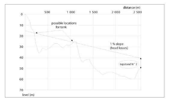
Figure 11.12: Selection of tank location (example of Aloua system).
