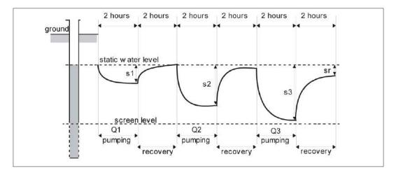
Figure 6.5: Well test with non-connected steps.
