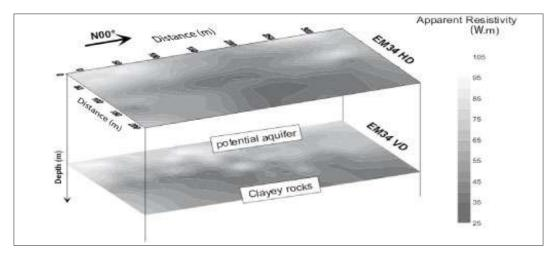
Figure 5.41: Apparent isoresistivity map (ACF, Uganda, 1999). EM34 a = 20 m, 20-m steps.
