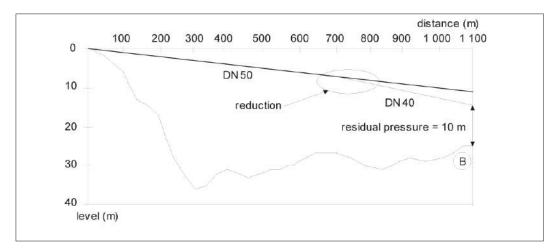
Figure 11.15: Combination of two pipe diameters to obtain a residual pressure of 10 mWG at Point B (example from first part of Aloua system).
