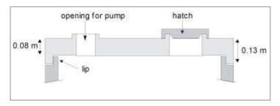
Figure 28: Well cover and inspection hatch.
