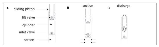
Figure 9.25: Working principle of a piston pump.
