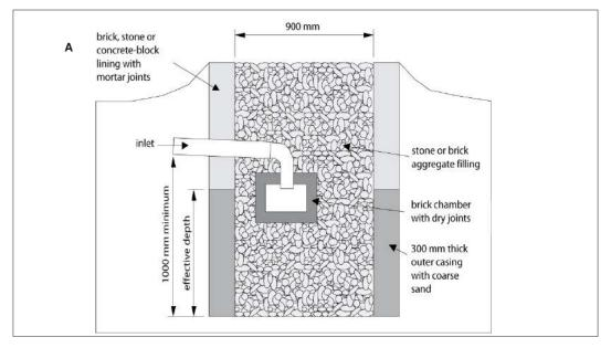
Figure 13.16: Soakaway pits. A: unlined pit.
