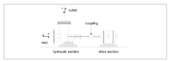
Figure 9.1: Electric centrifugal pump (surface).
