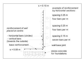
Figure 18: Example of reinforcement for a circular tank.
