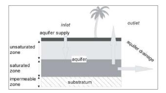
Figure 3.7: Storage and flow in an unconfined aquifer.
