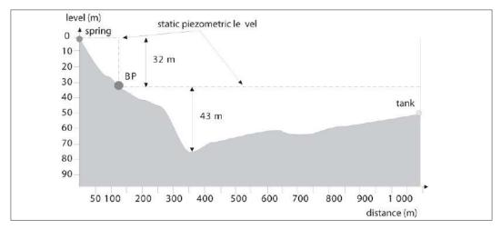
Figure 11.8: Installation of a break-pressure tank to stay within a pipe class (P<sub>static</sub> < 60 mWG).
