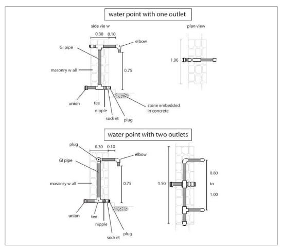
Figure 10.13: Plumbing for water point.
