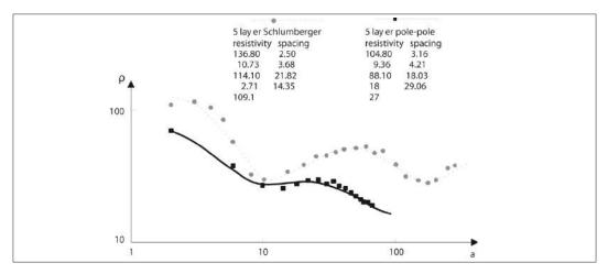
Figure 5.17: Example of a pole-pole survey (ACF, Siem Reap, Cambodia, 1998).
