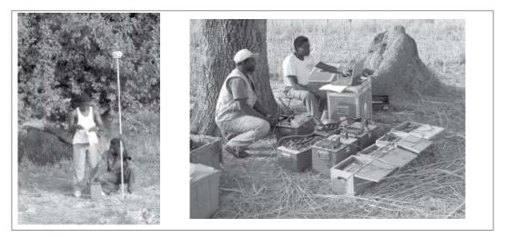
Figure 5.49: MRS equipment. A: geomagnetic field measurement using a proton magnetometer. B: Numis Plus equipment, ACF 2002.
