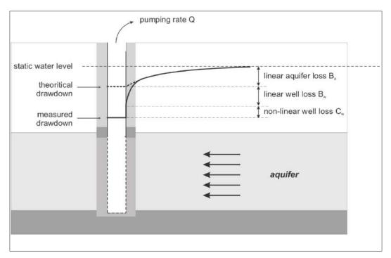
Figure 6.6: Various head-losses in a pumped well.
