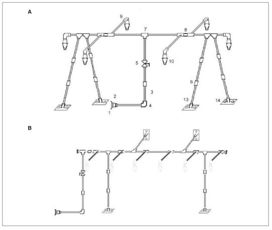
Figure 17.4: ACF tapstand kit. A: standard installation. B: installation against a wall.
