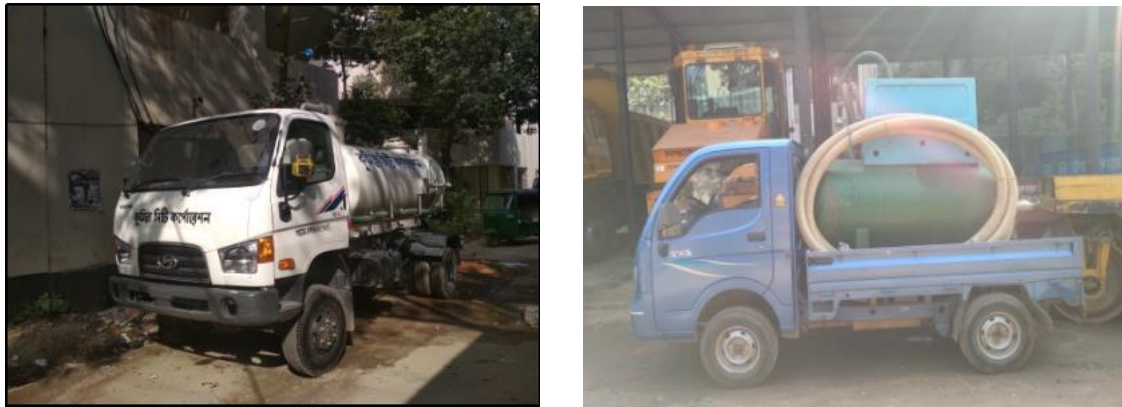
Figure 8: Septic tanks and pit emptying vehicle (vacuum truck) in Cumilla City Corporation (Source: Feasibility study 2020-21/DPHE).
