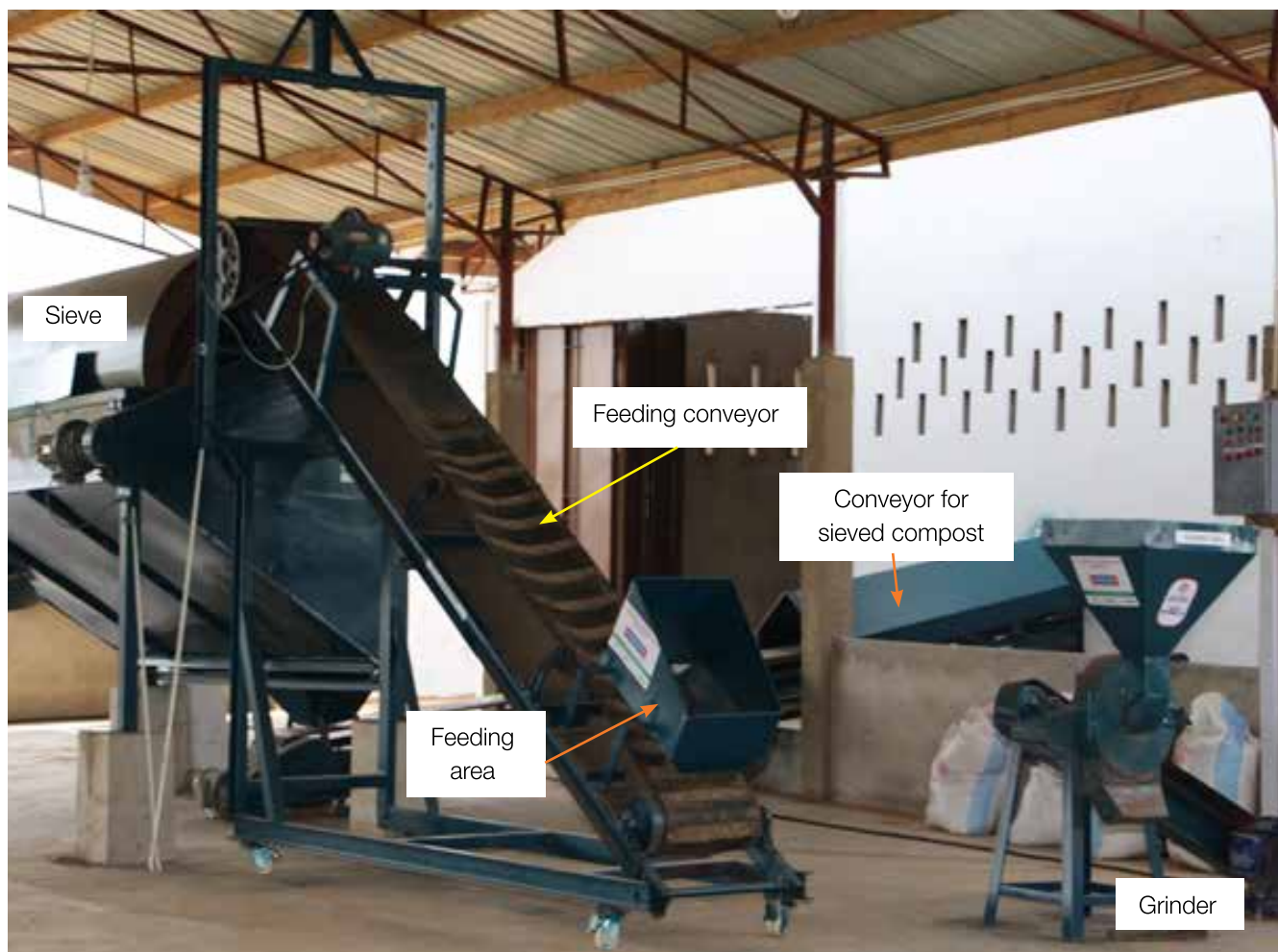
FIGURE 6. PROCESSING EQUIPMENT INSTALLED NEAR THE COMPOST MATURATION AREA AT THE FORTIFER PLANT IN GHANA.
