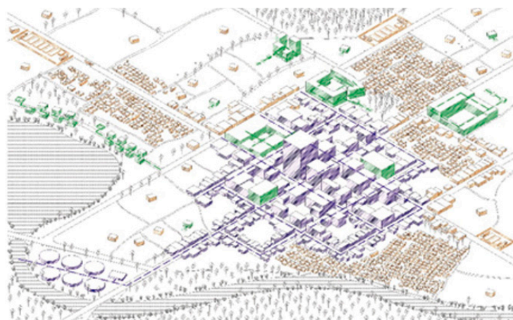
Fig. 1: Blended sanitation systems in urban settings (blue: sewerage, green: decentralised systems, brown: on-site sanitation). © Eawag-Sandec 2018
