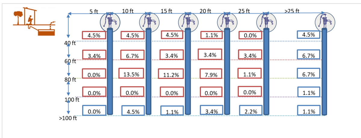
Figure 15: Depth of handpumps and lateral spacing of it with containment types lined tank with impermeable walls and open bottom (ENPHO, 2022).
