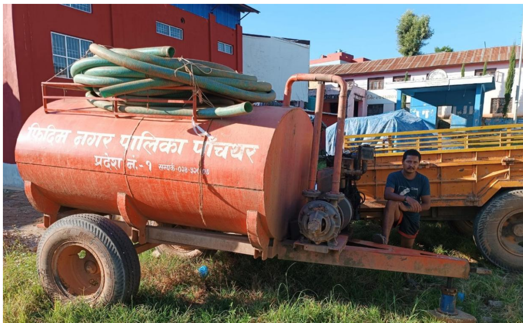
Figure 8: Mechanical Desludging Vehicle available in Phidim Municipality.
