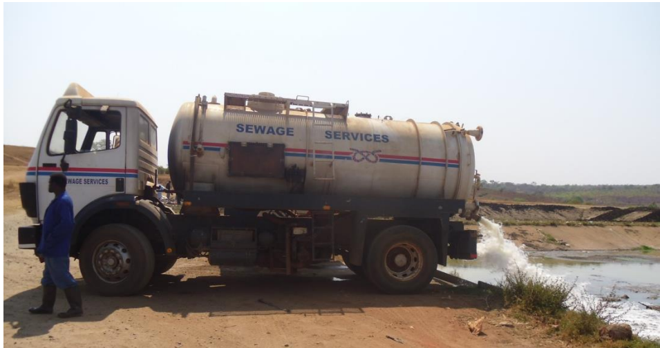
Figure 6: Vacuum truck emptying faecal sludge in a lagoon (Mkwezalamba and Kabika, 2023).
