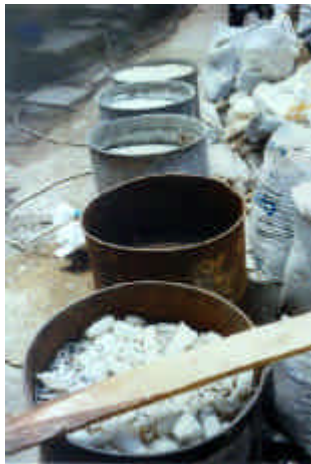
Figure 11: After washing and shredding different plastic fractions can be reused; Lima.
