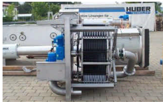
Figure 9: Container installation of a Vacuum Rotation UF-Membrane unit
