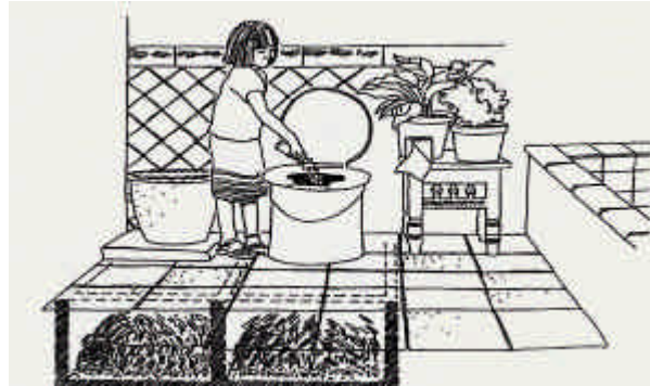
Figure 2: Dry, double-vault urine diversion toilet from Mexico.
