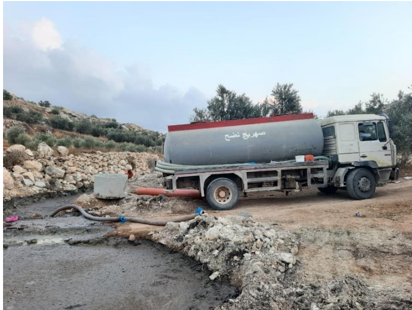
Figure 8: Truck discharging faecal sludge from septic tanks into a wadi.
