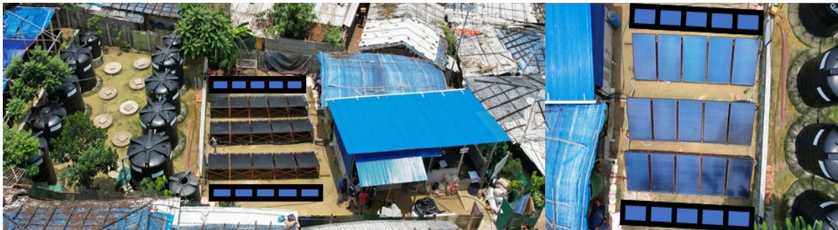
Figure 23. Possible aspect of the installation after adding 2 rows of 5 solar collectors (note: added collectors represented by a blue square)
